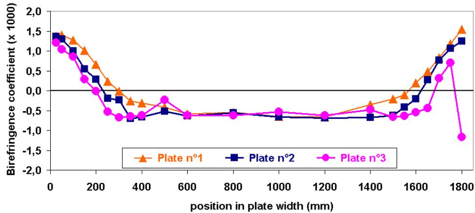
Fig. 5 - Birefringence coefficient evolutions measured across the width of three heavy industrial plates after a standardisation treatment. It displays a residual stress state across the width.
