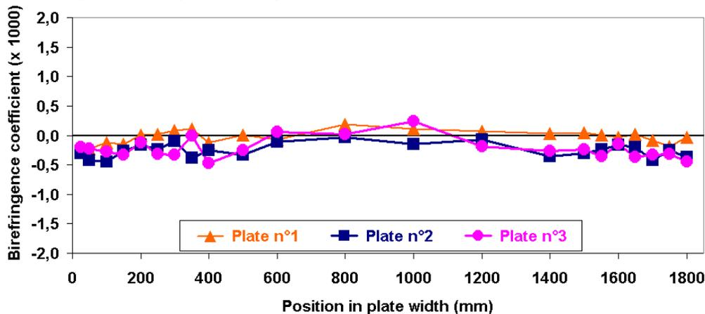
Fig. 6 - Birefringence coefficient evolutions measured across the width of same three heavy industrial plates, after a stress relieving heat treatment that minimised the residual stress gradients across the width.
