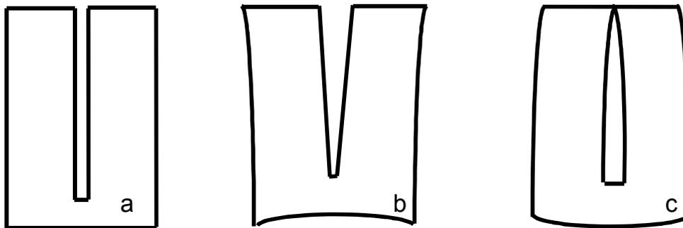
Fig. 1 - Different observable behaviours of heavy industrial plates during longitudinal splitting operation: a) the notch is linear without plate deformation, b) the notch opens up, c) the notch closes itself.
