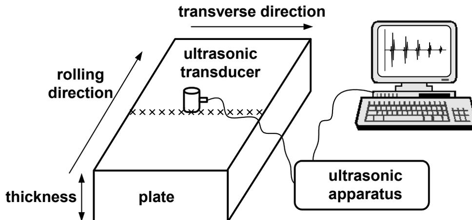
Fig. 2 - Schematic diagram of experimental apparatus used for birefringence coefficient determination. Crosses indicate the different measurement locations on heavy plates.
