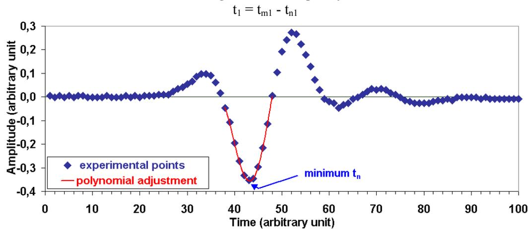
Fig. 3 - Determination of the back wall echo position by adjustment of a 4<sup>th</sup> degree polynomial on the first negative alternation of back wall echo and calculation of polynomial minimum  $t_n$ .
