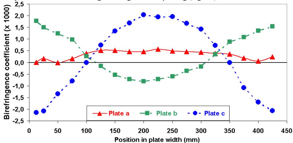
Fig. 4 - Different birefringence coefficient evolutions across the width of the three standard heavy plates, reflecting different residual stress states.
