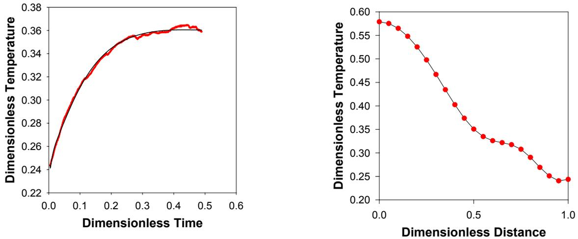
**Figure 3. a.** A typical plot of the measured temperature vs. time at one point on the surface of the preform and comparison with the predicted temperature. **b.** The initial temperature over the thickness of the preform just after it was taken out of the injection mold as reconstructed from the surface temperature data shown in Fig. 3a.
