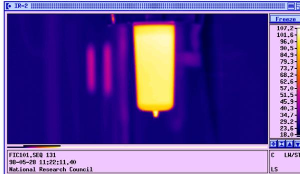
**Figure 2.** Shape and infrared image of the preform as it was taken out of the injection mold and held in place at the thread region.
