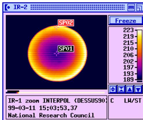
**Figure 4.** Infrared image of the billet top surface showing the surface-to-core temperature gradient resulting from the “skin effect” during induction heating.
