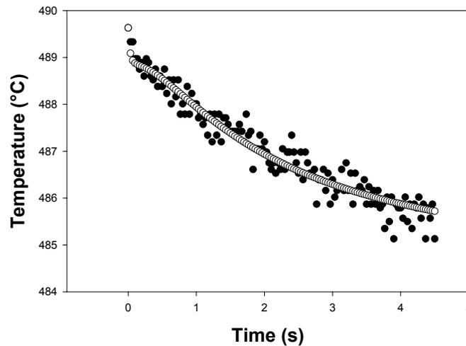
**Figure 6.** Comparison of the predicted temperature (o) at one point of the surface with the experimental data (●) measured with the infrared camera for the low-power experiment.
