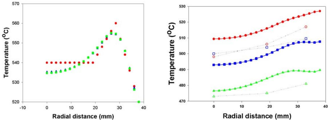
**Figure 5. a.** Comparison between the input initial temperature profile (○) and the reconstructed temperature profiles when the data are exact (□) and when the data contain 2% random noise (△). **b.** Recovered temperature profiles for the three power levels -High (○), Medium (□) and low (△)-. Temperature profiles measured with thermocouples for the three power levels -High (○), Medium (□) and low (△)-.
