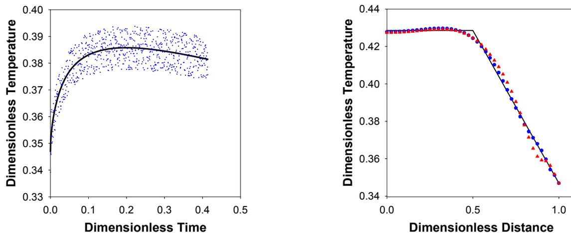
**Figure 1.** **a.** Surface temperature data generated numerically (exact (-), and noisy (+)) from an initial ramp function profile shown in Figure 1b. **b.** Comparison between the input initial temperature profile (-) and the reconstructed profiles when the data are exact (○) and when the data contain 2% random noise (▲).
