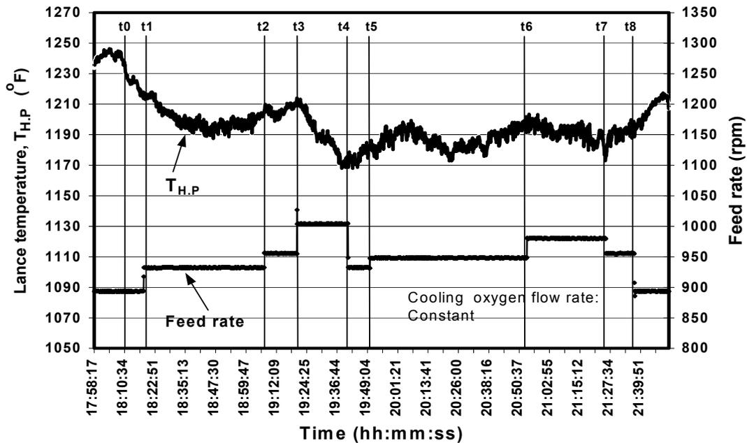
Figure 6: An oxygen lance as a temperature sensor in a lead recycling furnace
