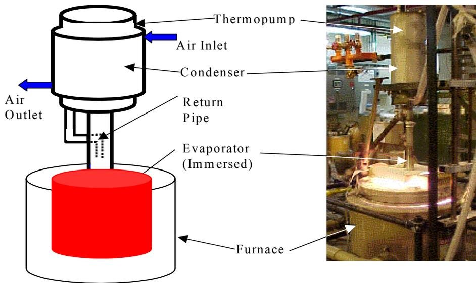
Figure 2: A schematic of a Thermopump
