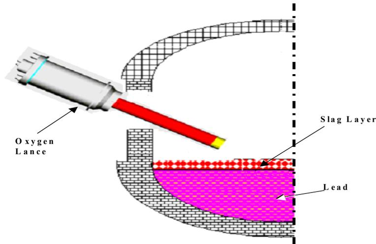
Figure 5: A schematic of an oxygen lance (Thermopump) in a lead recycling furnace
