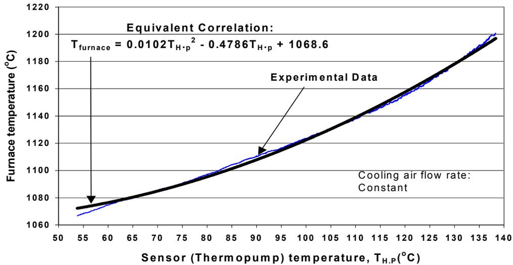
Figure 4: A Thermopump as a temperature sensor in a gas furnace
