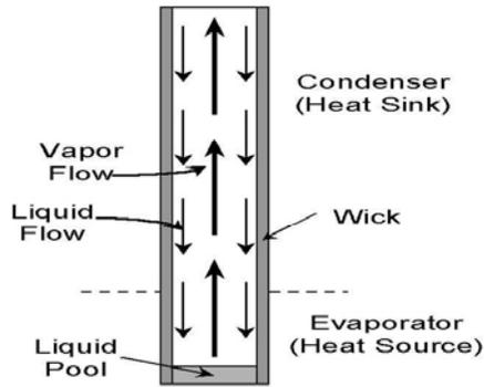
Figure 1: A typical vertical heat pipe
