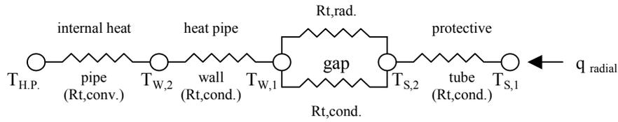
Figure 9: An equivalent thermal circuit for temperature sensor system
