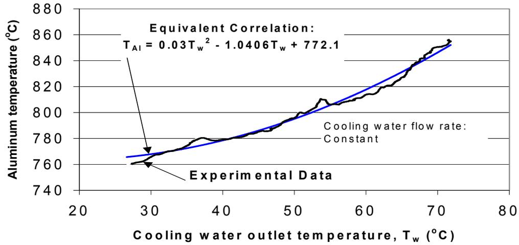
Figure 7: A Thermopump as a temperature sensor of molten aluminum
