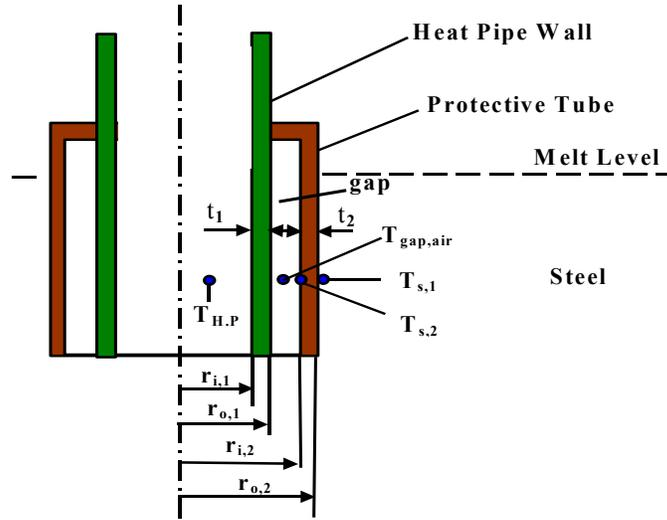
Figure 8: A schematic of temperature sensor system
