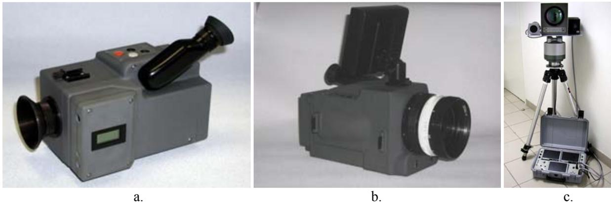
**Fig. 1. Thermovisors TN-4604MB (a), TN-4604MP (b) and TN-4604MP-100 (c)**
