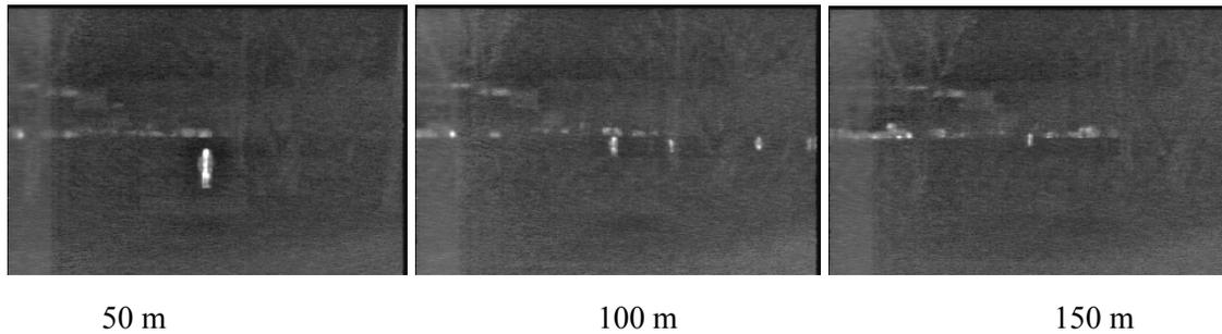
**Fig. 2. Images of person detected at various distance.**
