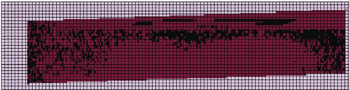
Fig.3. Thermogram of the thermoprotective coating with a defect (in the center) and noise caused by surface emissivity.
