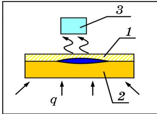
Fig. 1. Detachments in a thermoprotective coating: 1- coating, 2- substrate, 3-IRI imager.
