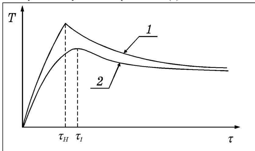
Fig.2. Surface temperature dependences on time for unfaulty (1) and faulty (2) parts of the structure.
