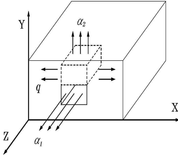
Fig. 4. Thermophysical model of the cooling passage in a turbine blade.
