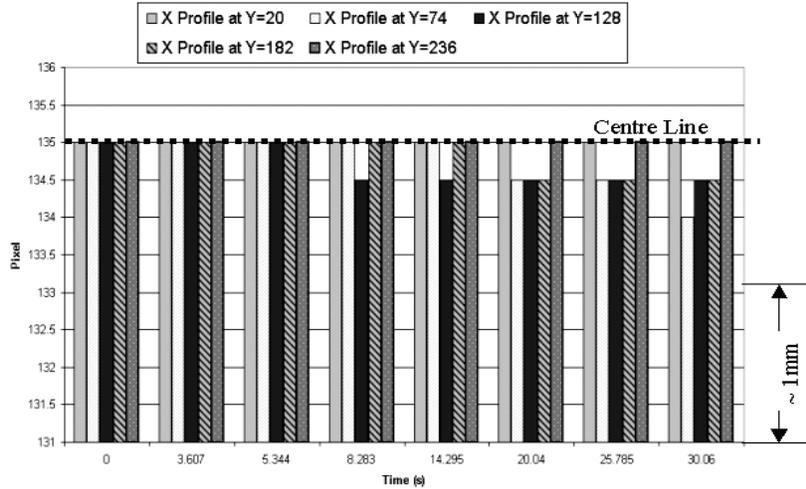
Figure 10: Pixel value of centre line of strut at positions along the length of the strut– vs.- transient time for 2mm thick CFRP skin and strut.
