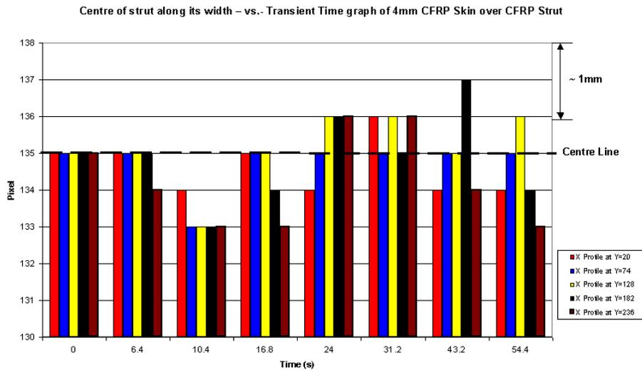
Figure 12: Pixel value of centre line of strut at positions along the length of the strut– vs.- transient time for 4mm thick CFRP skin and strut.
