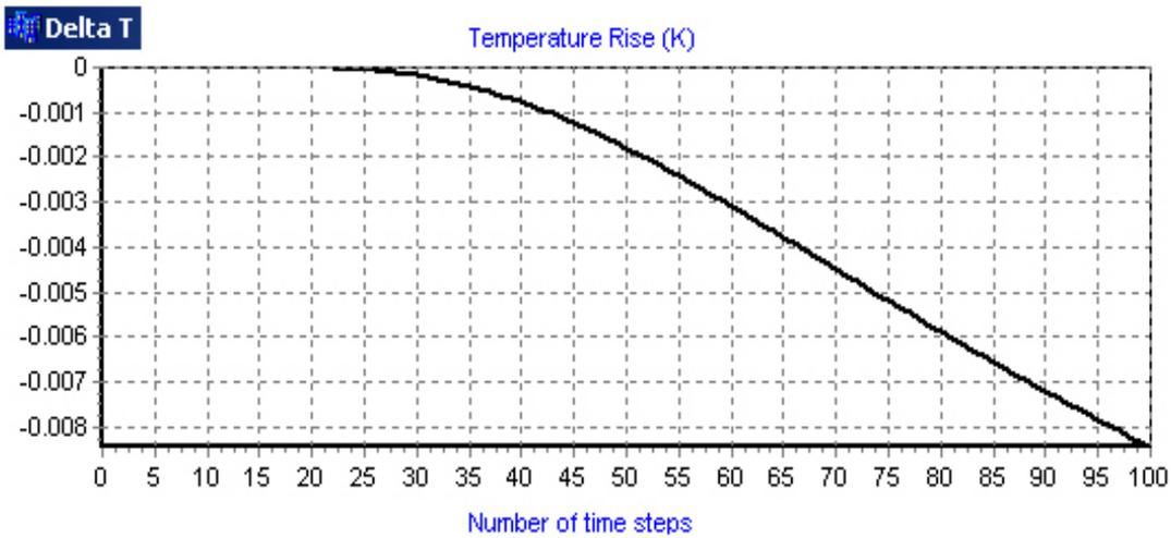
Figure 5: Modelling: thermal contrast vs. Time plot of 4mm CFRP skin over CFRP strut
