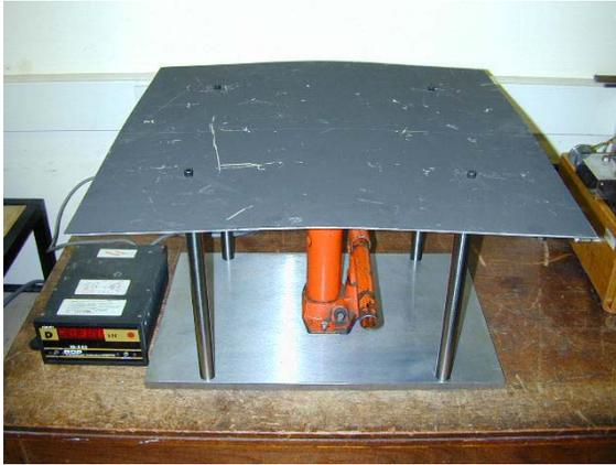
Figure 2: Test rig used to apply a load to a strut beneath a skin.
