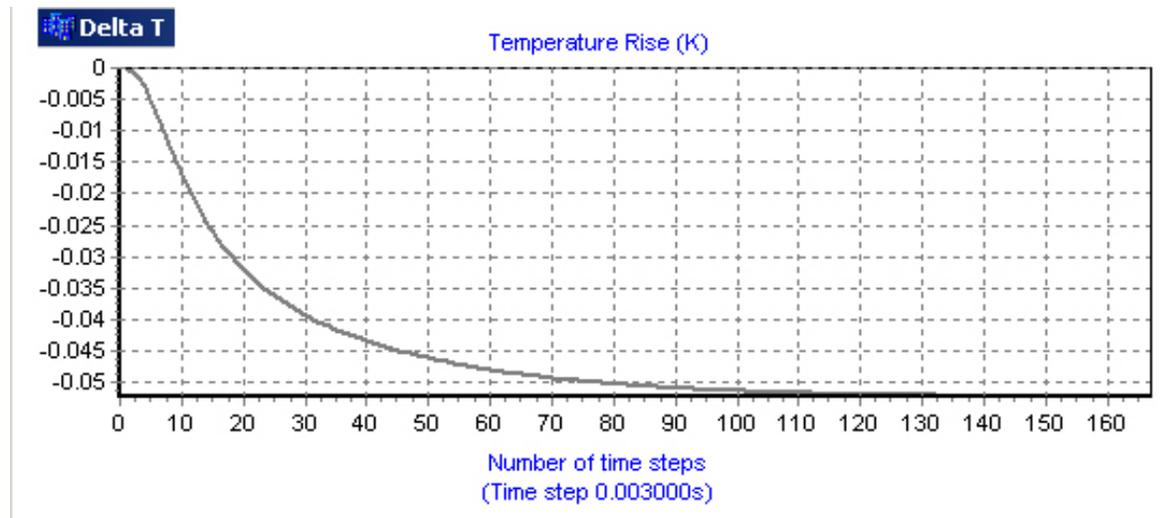
Figure 3: Modelling: thermal contrast vs. time plot of 1.6mm Al alloy skin over Al alloy strut.
