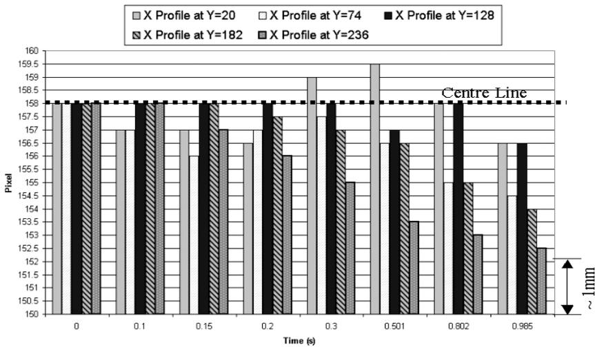
Figure 8: Pixel value of centre line of strut at positions along the length of the strut- vs.- Transient Time for Al panel in the 5cm bending condition.
