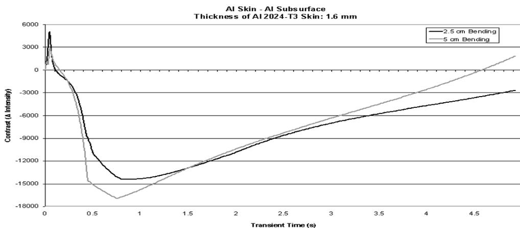
Figure 7: Thermal contrast curves of Al panel
