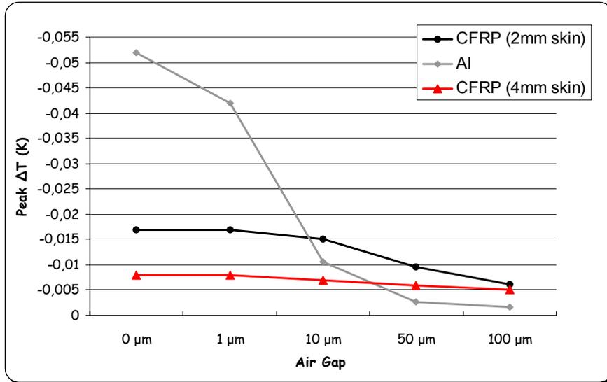
Figure 6: Modelling: peak  $\Delta T$  against air gaps for CFRP and aluminium panels
