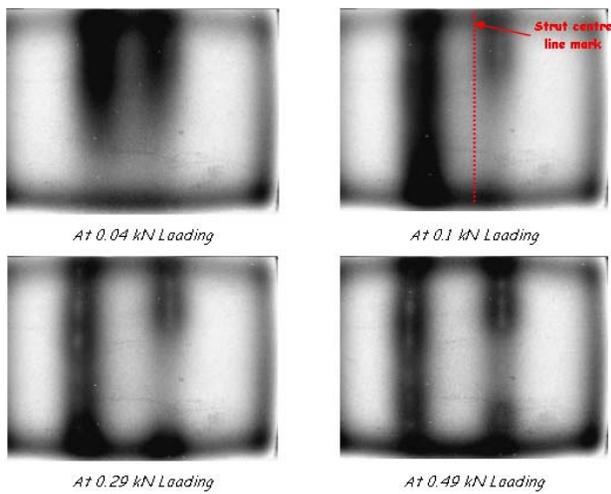
Figure 9: Thermal images for Al panel in the 5cm bending condition.
