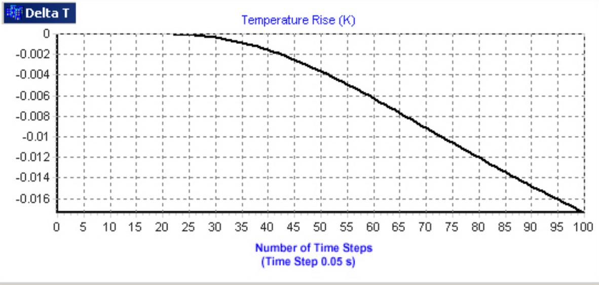
Figure 4: Modelling: thermal contrast vs. time plot of 2mm CFRP skin over CFRP strut
