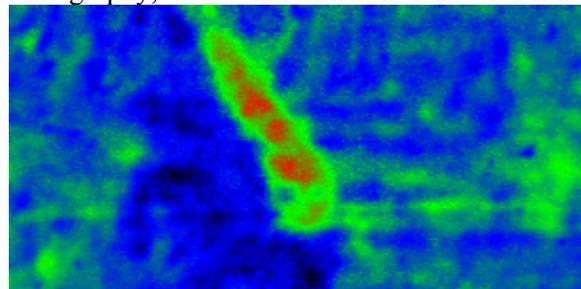
Fig. 3d: *phase* map as produced by PPT performed using the same raw data
