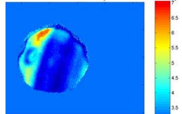
Fig.7b: thickness map, mean diffusivity value:  $4.77 \cdot 10^{-7} \text{ m}^2 \text{ s}^{-1}$
