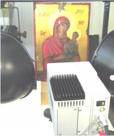
Fig.6a: Pulsed Thermography set up inspecting a wooden painting (photographic flashes and FPA IR camera)
