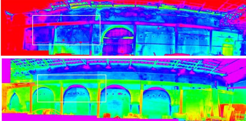
Fig. 1a: Moisture monitoring by statistical analysis of the historical arsenal of Venice (*Tezone 105*): thermograms of internal walls (top West, bottom East), the marked areas have been composed on fig.1b
