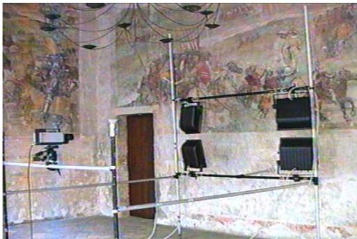
Fig. 3a: experimental set up for the Romanino's fresco delamination testing (Malpaga castle)
