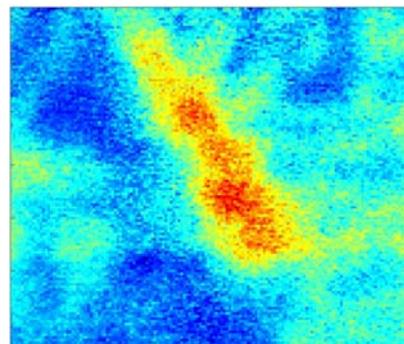
Fig. 3b: *timegram* as produced by Thermal tomography, corrected for the 3D heat diffusion
