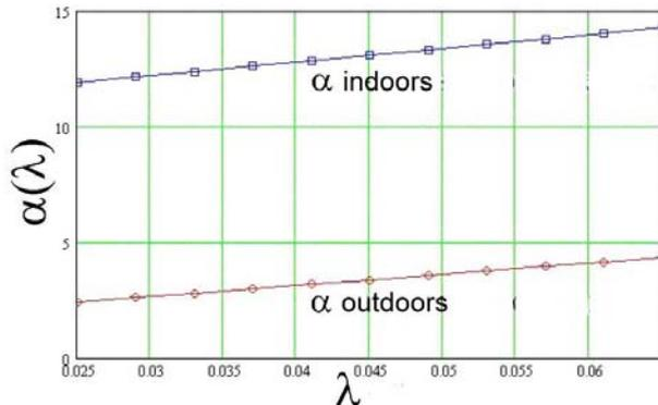
Fig. 3. Outdoor structure's heat emission factors of the inner (with given value 3.7) and outer (given value 13.7) surfaces with their dependency of the heat conductivity, calculated using (12). Probability functional for this case is presented at fig. 2.
