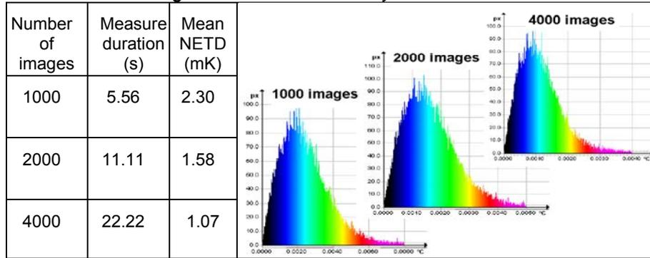
**Fig. 3. NETD enhancement by lock-in detection (1 Hz): influence of the number of images accumulated**
