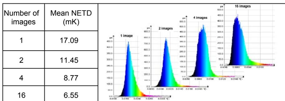
**Fig. 2. NETD enhancement by time accumulation and influence on the histogram**
