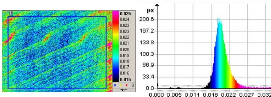
**Fig. 1.** Distribution (left) and histogram (right) of the pixel standard deviation calculated from 256 images of an extended blackbody at 20°C, for a field of 320x240 pixels, an image rate of 180 Hz and an integration time of 400  $\mu$ s. The NETD is assimilated to the mean value of the standard deviation for the full image.
