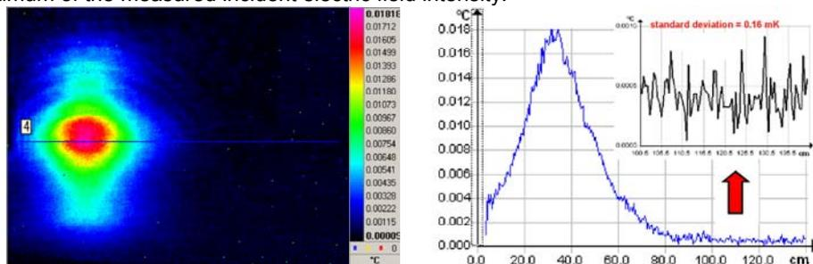
**Fig. 5.** NETD evaluation in the EMIR measurement conditions. Left: EMIR lock-in image of the electric field intensity. Right: horizontal profile and part of it used for evaluation of the NETD (assimilated to the space noise standard deviation).
