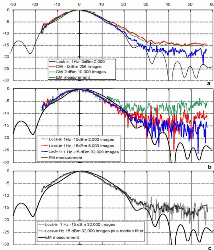
**Fig. 4.** Comparison between CW and square-modulated emission and their respective time and frequency data processing. a) CW measurements with time accumulation and lock-in detection, for a power of 0 dB. b) Influence of the number of images processed by lock-in detection (power: -15 dBm). c) Mixing space and frequency data processing with square-modulated emission (power: -15 dBm).
