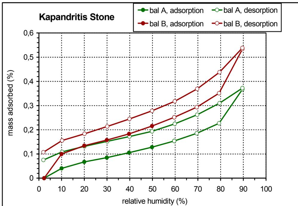
Figure 7: Isothermic curves of Kapandritis stone samples
