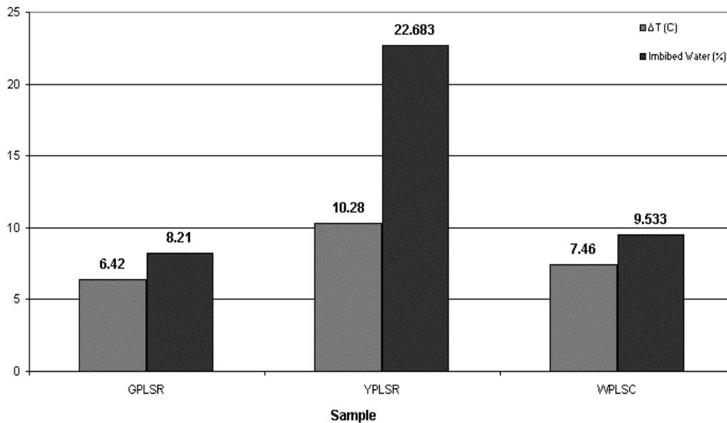
Figure 4:  $\Delta T$  and Imbibed Water % of investigated porous stones after the capillary rise tests
