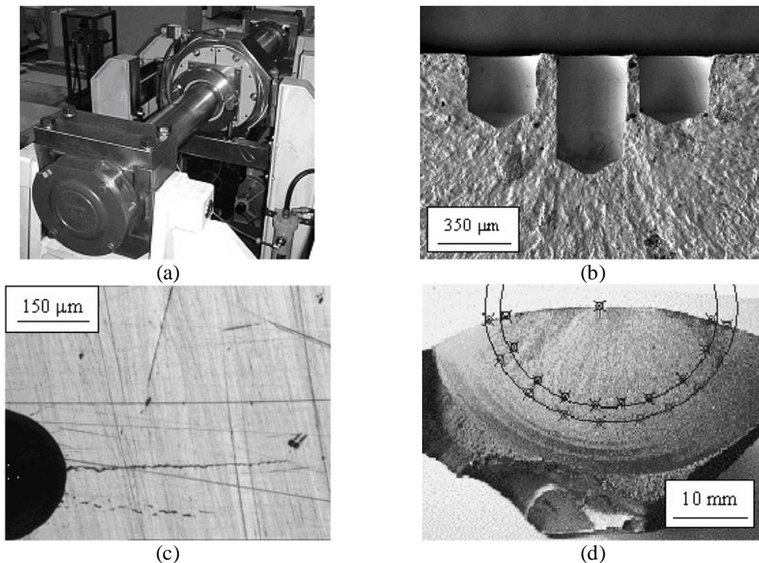
Figure 1 – Details of full-scale experiments on railway axles: a) the test rig; b) micro-holes on a full-scale specimen; c) an example of the axle surface during a propagation test; d) analysis of the crack shape evolution.
