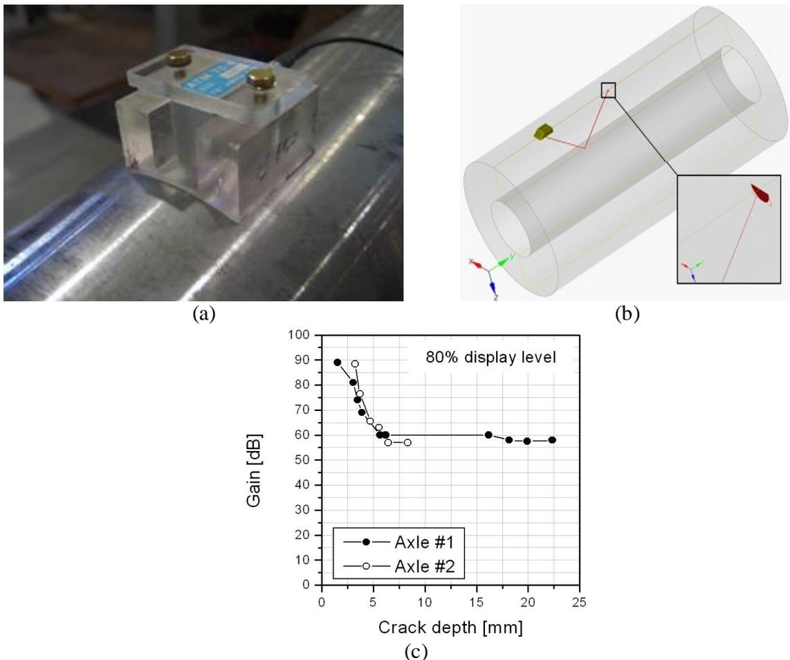
Figure 2 – UT measurements of a developing fatigue crack: a) wedge in plexiglas; b) schematic of the “2<sup>nd</sup> leg” inspection; c) resulting dB-depth curves.
