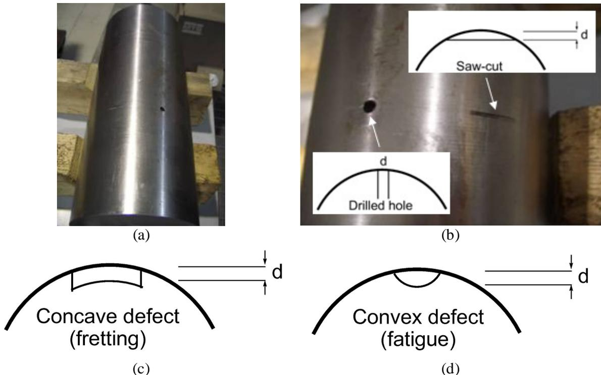
Figure 3 – Notches considered for the analysis: a) sample block with saw-cuts and drilled holes; b) detail of the same block; c) concave EDM notches; d) convex EDM notches.
