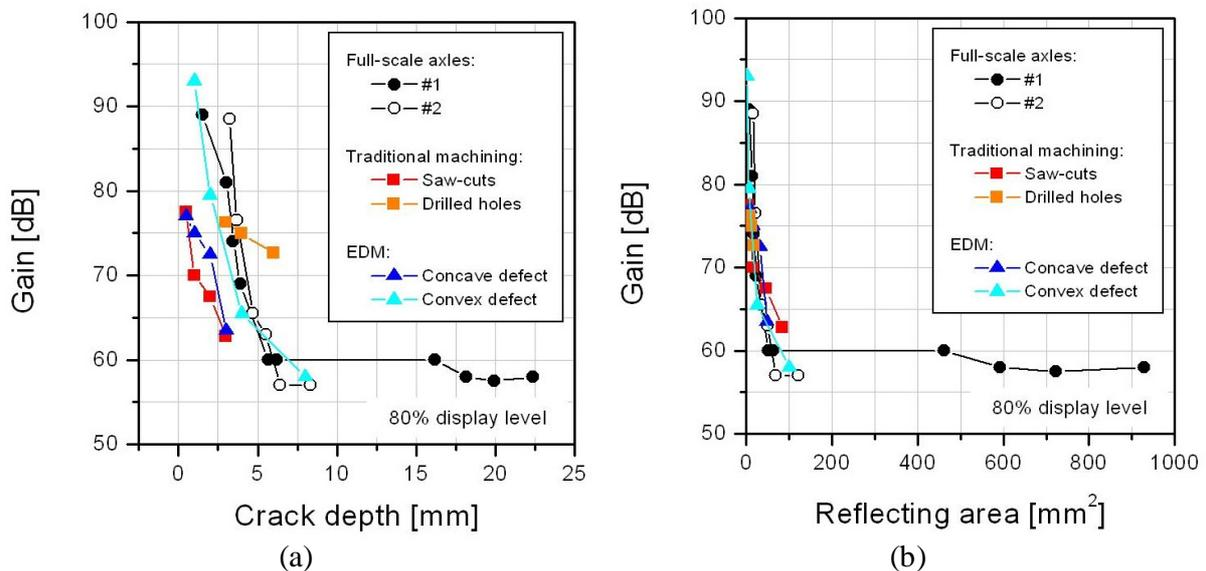
Figure 4 – Cracks and notches responses in terms of crack depth (a) and reflecting area (b).
