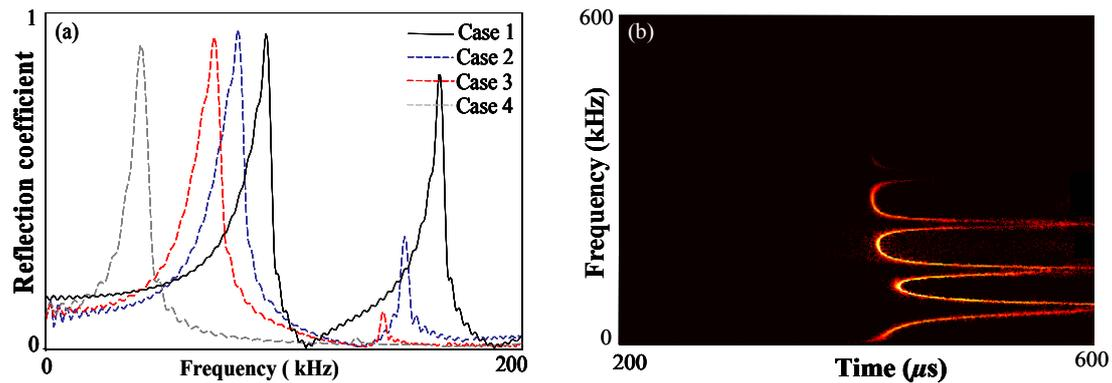
**Figure 5** (a). Reflection coefficient spectrum obtained from the pipe with imperfectly bonded blockage layers. (b). Reassigned Spectrogram analysis of the transmitted signal in the pipe with imperfectly bonded blockage layer (case 2).
