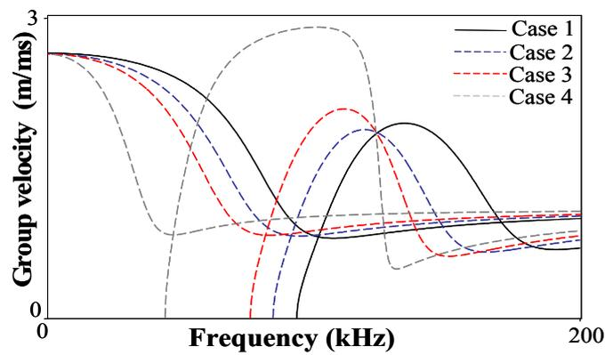
**Figure 4.** Dispersion curves of the torsional modes in the bilayered pipe with different bonding states. (case 1:  $K_T \in \infty$ , case 2:  $K_T = 3.5 \times 10^{18} \text{ N / m}^3$ , case 3:  $K_T = 1.75 \times 10^{18} \text{ N / m}^3$ , case 4:  $K_T = 3.5 \times 10^{17} \text{ N / m}^3$ ).
