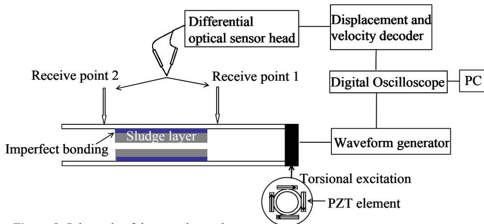
**Figure 8.** Schematic of the experimental setup
