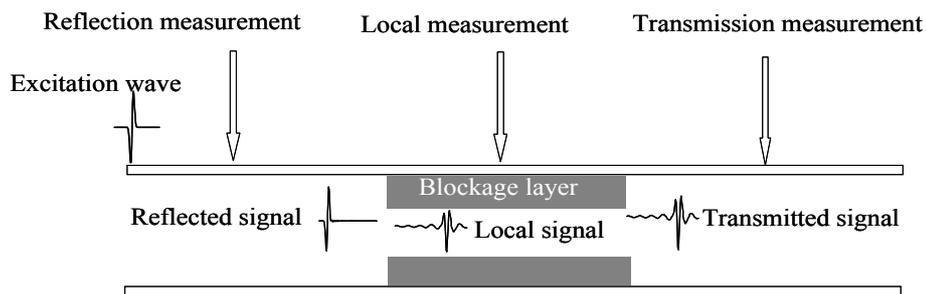
**Figure 1.** Schematic of the idealised model of a pipe with a sludge layer.
