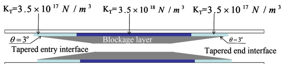
**Figure 6.** Schematic of the pipe with the sludge that has varying thickness and bonding state
