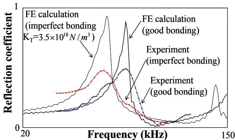
**Figure 9.** Reflection coefficient measured at point 1 from the samples with good bonding and imperfect bonding.
