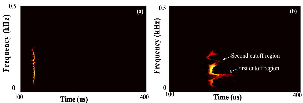
**Figure 10.** (a) Reassigned Spectrogram of the incident signal before the blocked pipe region (measured at point 1). (b) Reassigned Spectrogram of the transmitted signal after the blocked pipe region (measured at point 2).
