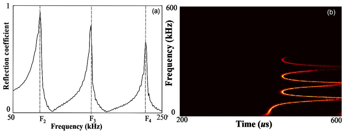
**Figure 3** (a). Reflection coefficient spectrum of the bilayered pipe. (b). Reassigned spectrogram analysis of the local signal in the bilayered pipe.
