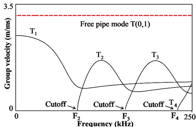
**Figure 2.** Group velocity dispersion curves of torsional modes in the free (red line) and the bilayered (black curves) pipe (simulated by DISPERSE1).
