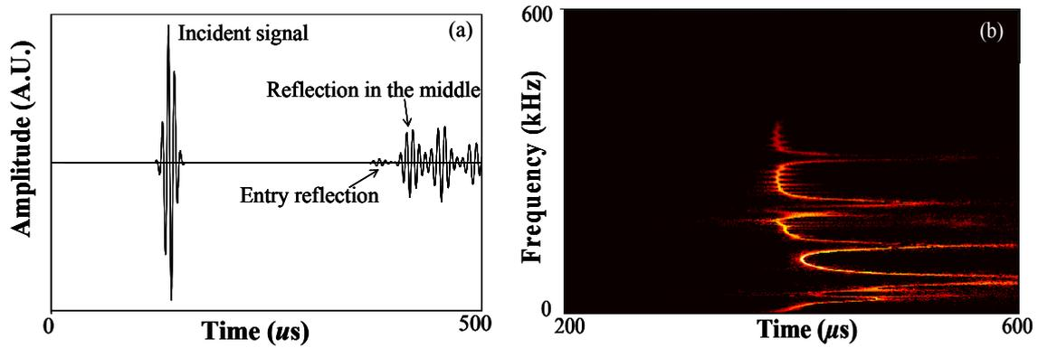
**Figure 7** (a). Time trace of the incident signal and the reflected signals in the pipe with blockage layer of varying thickness and bonding state. (b). Reassigned Spectrogram analysis of the transmitted signal in the pipe with blockage layer of varying thickness and bonding state.
