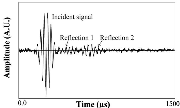
**Figure 11.** Time trace of the incident signal and the reflected signals measured at point 1.
