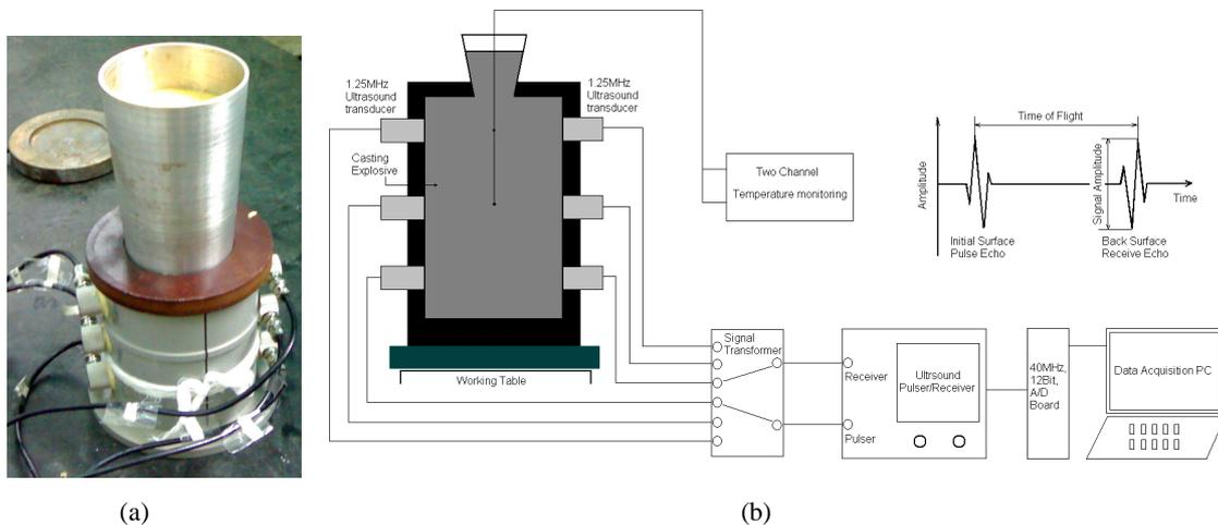
Fig.1 Schematic diagram of the molding device (a) and ultrasonic measurement (b)
