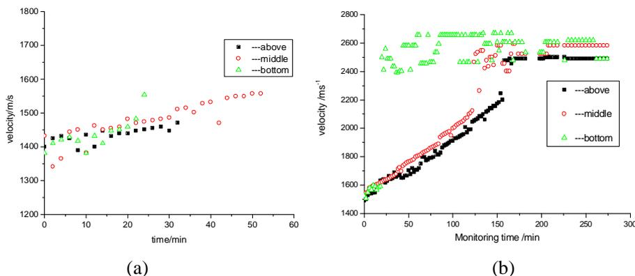
Fig.3 The ultrasonic velocity along with freezing time (a) TNT (b) TNT mixture explosive
