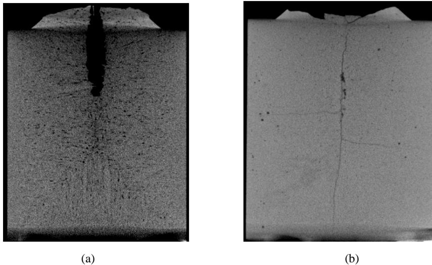
Fig.5 CT images of inter structure of explosive after solidification. A great deal of interspaces are produced in TNT explosive (a) and crack is produced in TNT mixture explosive (b)
