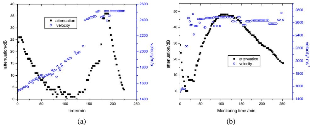
Fig.6 The ultrasonic velocity and attenuation trend along with solidification (signals from sensors above (a) and underside (b))
