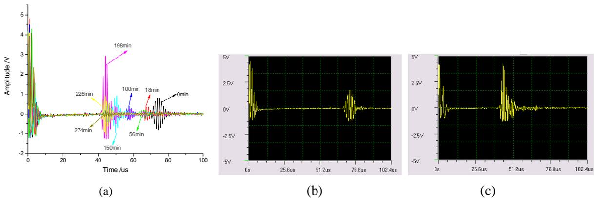
Fig.2 The change characteristic of waveform (a) typical waveform at starting (b) and at the solid-liquid border (c)
