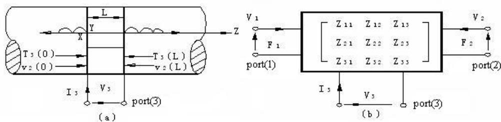
(a) Geometrical model for transducer
