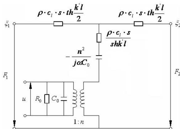
Figure 2 Mason equivalent circuit of piezoelectric crystal
