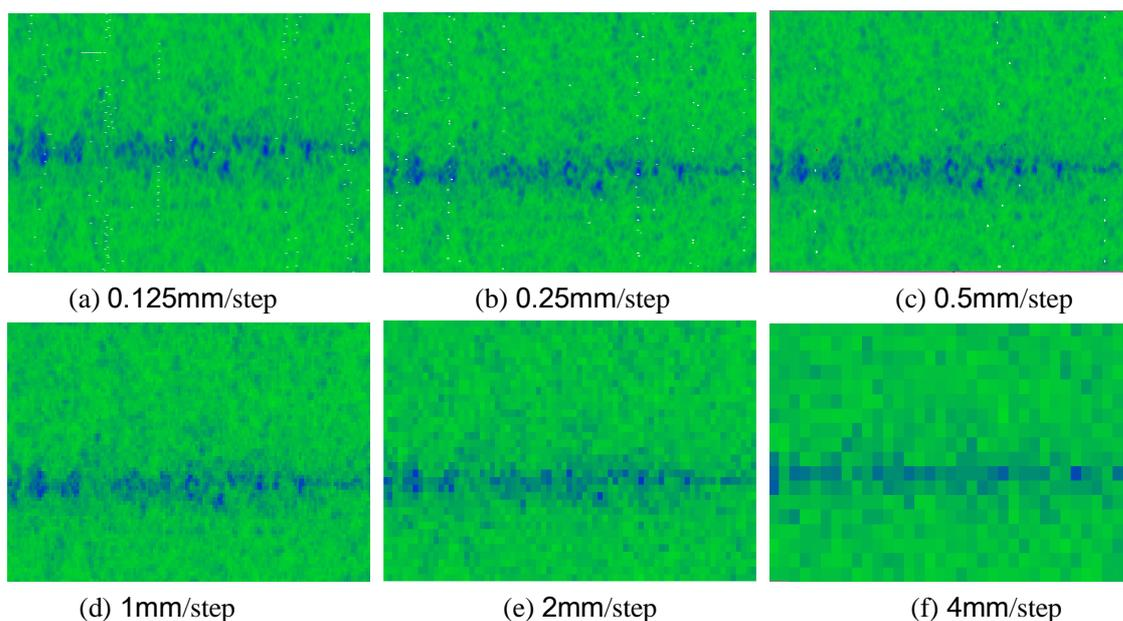
Fig 3. The C-scan results on the same area where inclusions were detected with different scanning steps
