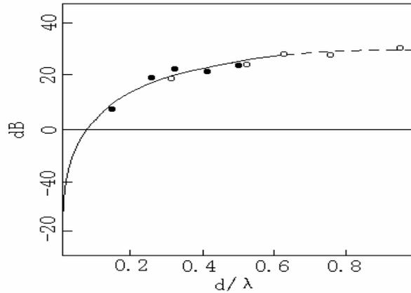
Figure 1 The relationship between echo amplitude and  $d/\lambda$  based on the detection experiment on 0.5mm bottom hole drilled in the bottom side of the normalized Ni-Cr-Mo alloy steel specimen by B4S and B2S transducers (● 2MHz, ○ 4MHz)
