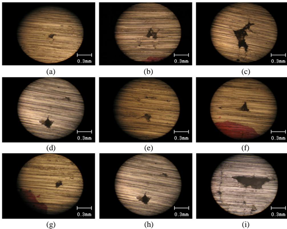
Fig 5. The morphology of 9 dissected inclusions after slab specimen was dissected by grinding machine.
