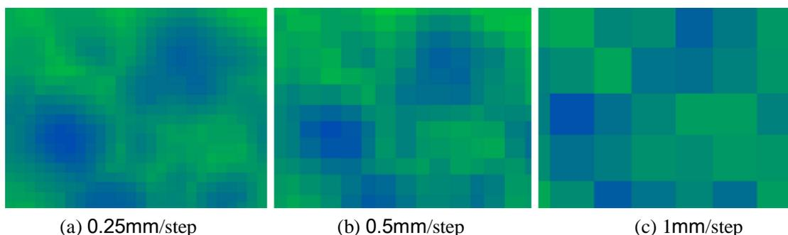
Fig 4. The detailed images of the same region within the scanned specimen of different scanning step.
