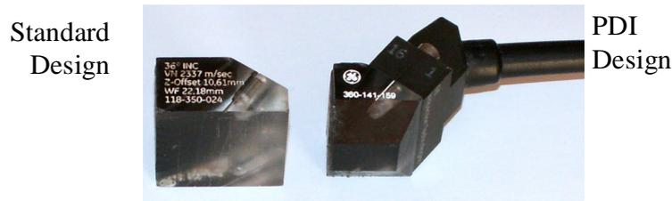
Figure 4. Standard Wedge versus PDI Wedge
