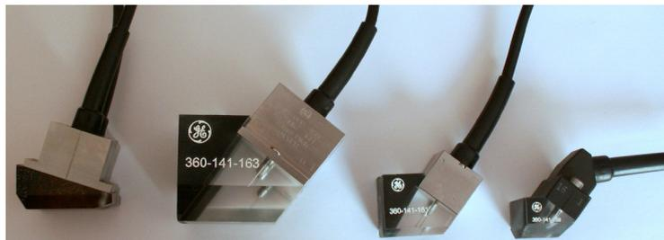
Figure 2. Linear Phased Array probes
