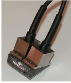
Figure 3. Dual Matrix Probe
