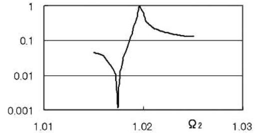
Fig. 6 Reflection coefficient
