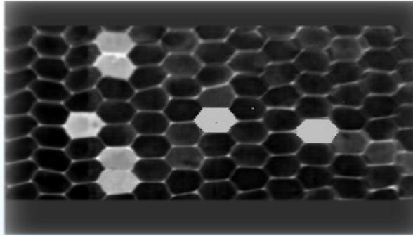
**Fig.3 computed radiograph of water in honeycomb structure**
