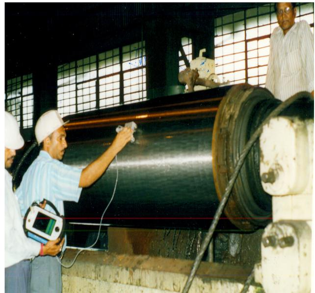
Fig. 2- ICDP work roll being tested manually with hand held eddy current testing instrument
