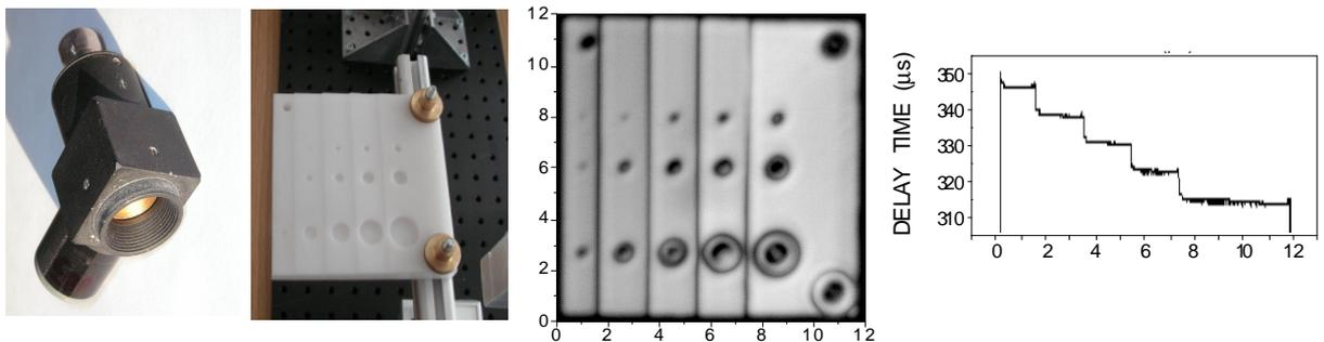
Fig. 2: From left to right: EMFI transducer, sample under test (step wedge), 2D-scan (scanning area is 12 cm x 12cm) as function of delay time, line scan of delay time shows sharp steps.
