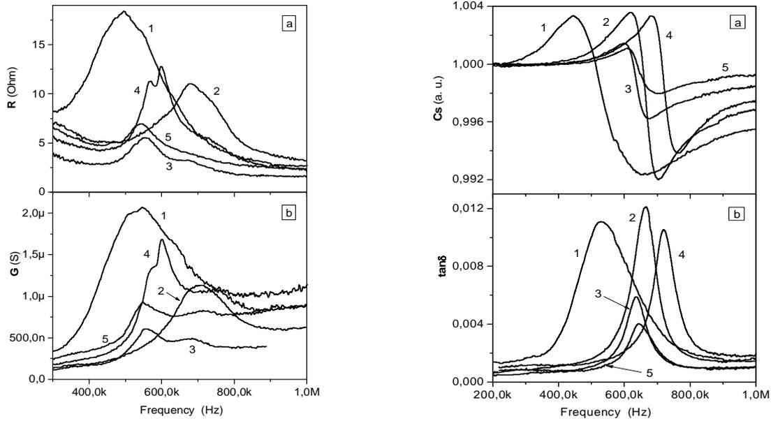
Fig. 1. Comparison of the EMFIT films with different evaporated electrodes.  $C(f)$ ,  $\tan\delta(f)$ ,  $R(f)$ , and  $G(f)$  as function of the operation frequency. Sample no. (1) – (5) denote the different films according to tab.1. Left: Films without embedding them into the sensor, right: Film was embedded into a sensor.
