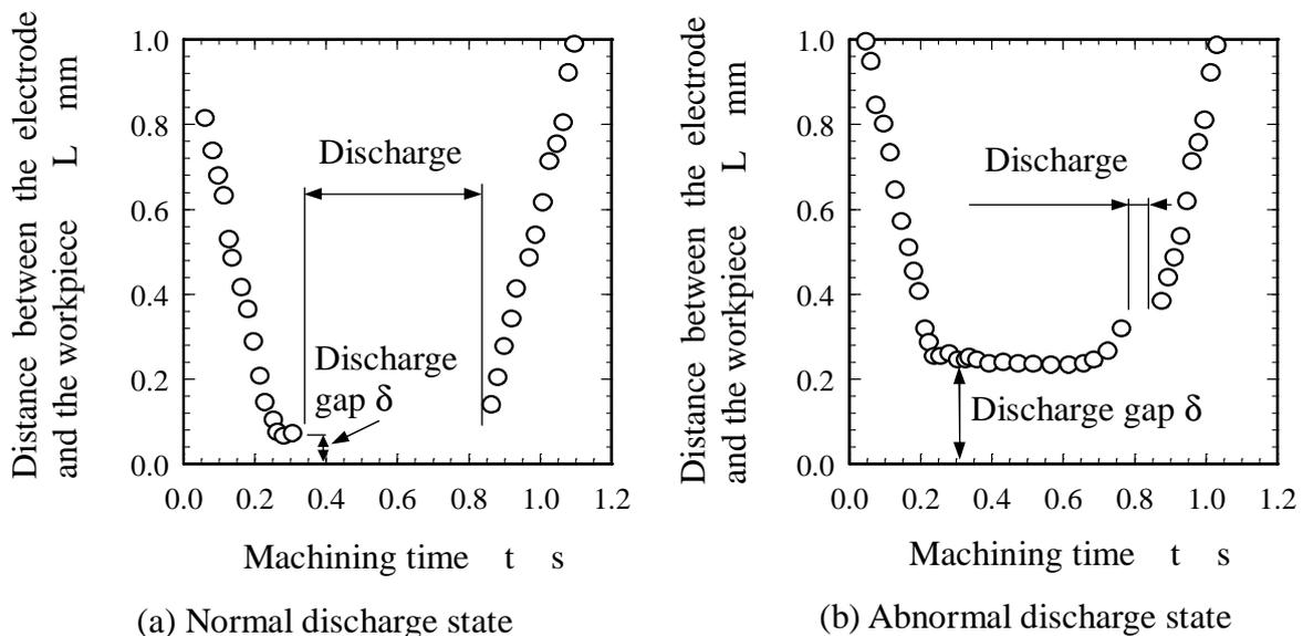
Fig.2 Discharge gap
