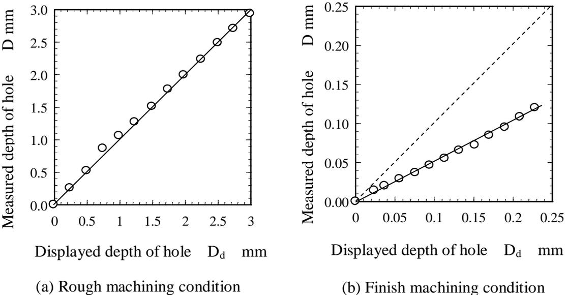
Fig.3 Relationship between the displayed depth of hole and measured one
