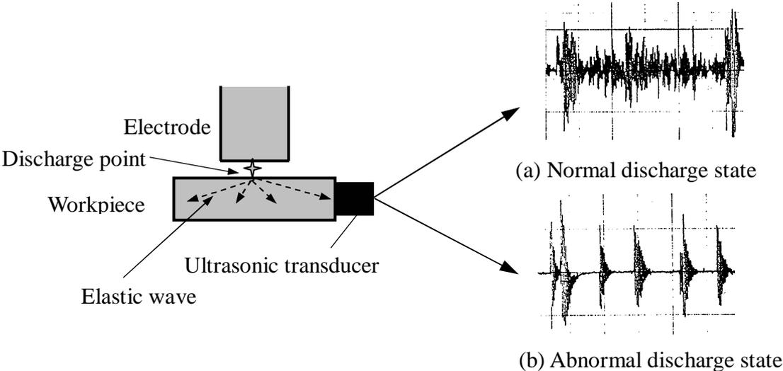
Fig.4 Received elastic waves
