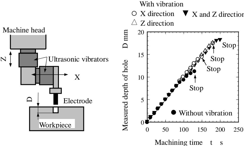
Fig.5 Electric discharge with the ultrasonic vibration
