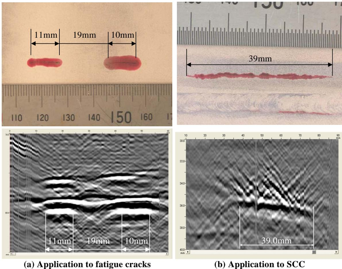
Figure 9. Application results to cracks
