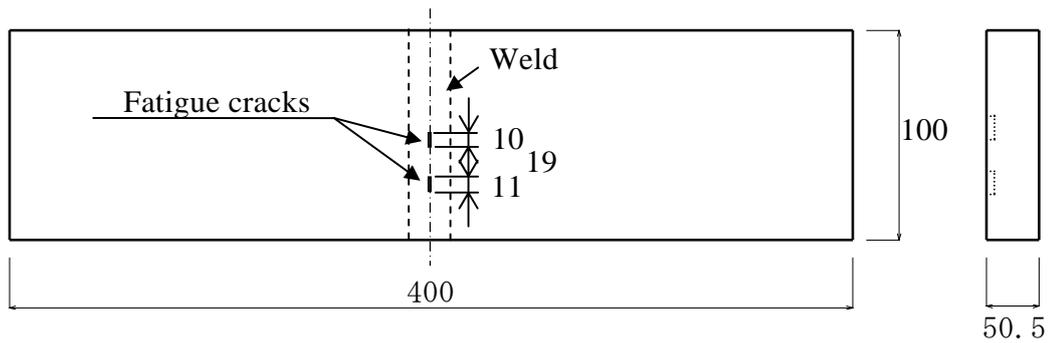
**Figure 5. Test specimen in which fatigue cracks are implanted**
