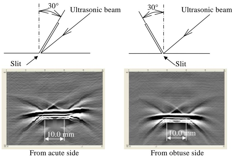
Figure 8. Application results to the tilted slit
