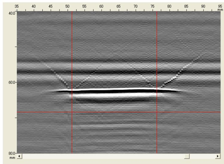
**Figure 3. Example of the image of Twin Diffraction Waves Technique (Actual length: 25.0mm, UT result: 25.0mm)**
