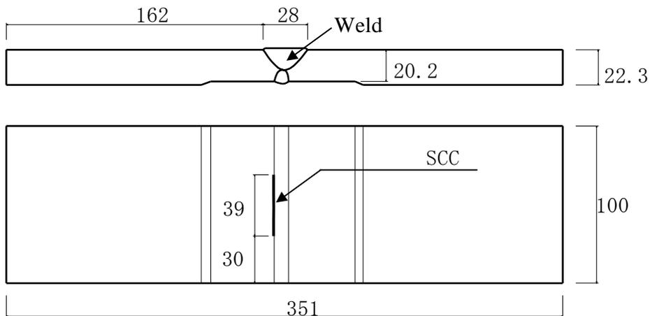
**Figure 6. Test Specimen with SCC**
