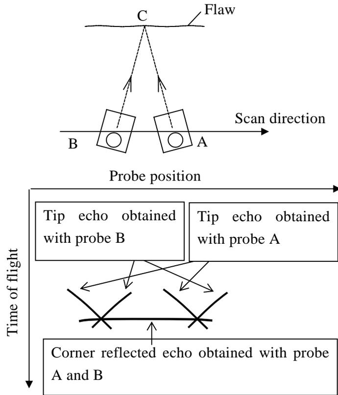
**Figure 2. aRelation between the position of probes and the propagation time of the diffraction wave from the edge of the flaw**
