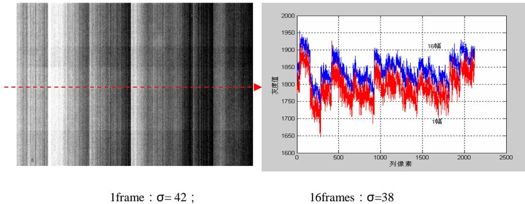
The gray curve of Figure 1 shows that the standard deviation of the image has a small decline after the 16 image are stacked, that is, system noise suppression is not obvious at this time, the nonuniformity of the system is more than random noise for the impacting of the system image quality. So it is the primary problem that eliminates inconsistencies for the optimization of system image quality.
