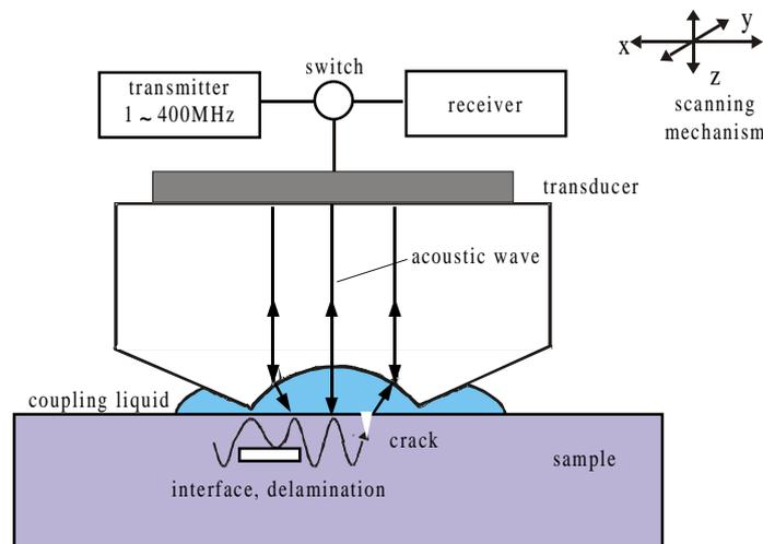
Fig.2 Working principle of SAM
