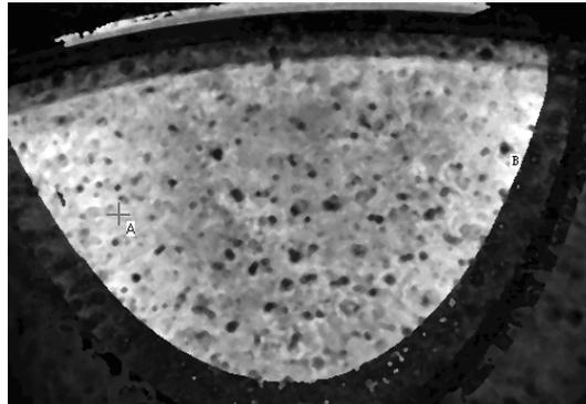
d) SAM image of Aluminum alloy/interstice interface: formed by the second reflection wave in fig. 6 b)
