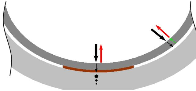
Fig.3 Ultrasonic transmission and reflection in typical parts of the binding
