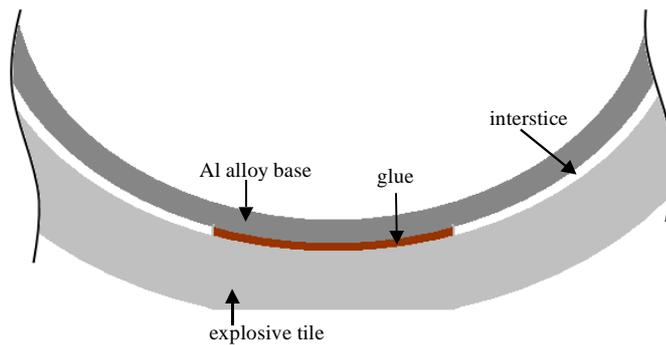
Fig.1 Structure of the binding
