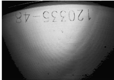
c) SAM image of water/Aluminum alloy interface : formed by the first reflection wave in fig. 6 b)
