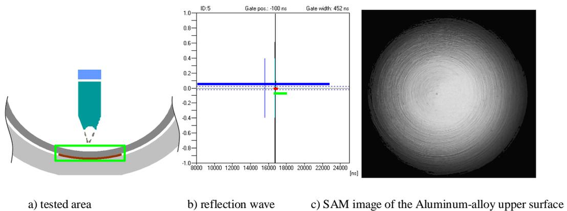
Fig.6 Results tested for central area of binding by SAM
