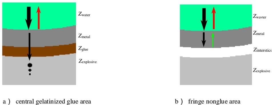
Fig.5 Ultrasound reflection and transmission in binding
