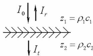
Fig.4 Reflection and transmission of vertical incident wave at interface
