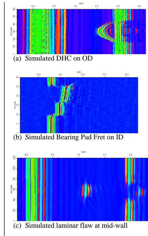
Figure 7: B-scan images of simulated flaws in pressure tube
