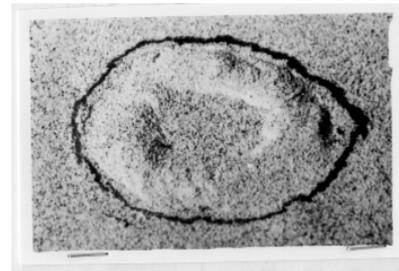
Figure 2: IGSCC generation in laboratory
