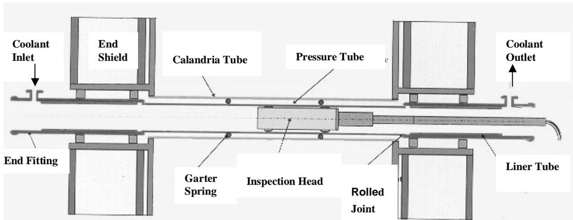
Figure 3: Typical PHWR coolant channel assembly
