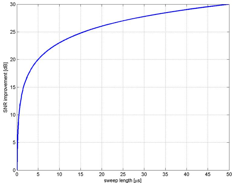
**Figure 5 Improvement of the signal to noise ratio as function of sweep length. For relatively short sweeps improve the signal to noise ratio very efficiently.**
