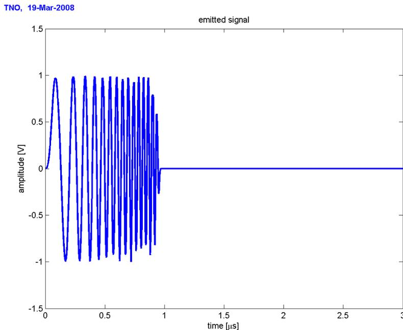
**Figure 2 Initially emitted excitation signal, which is a short sweep. In this sweep the frequency is gradually increased.**
