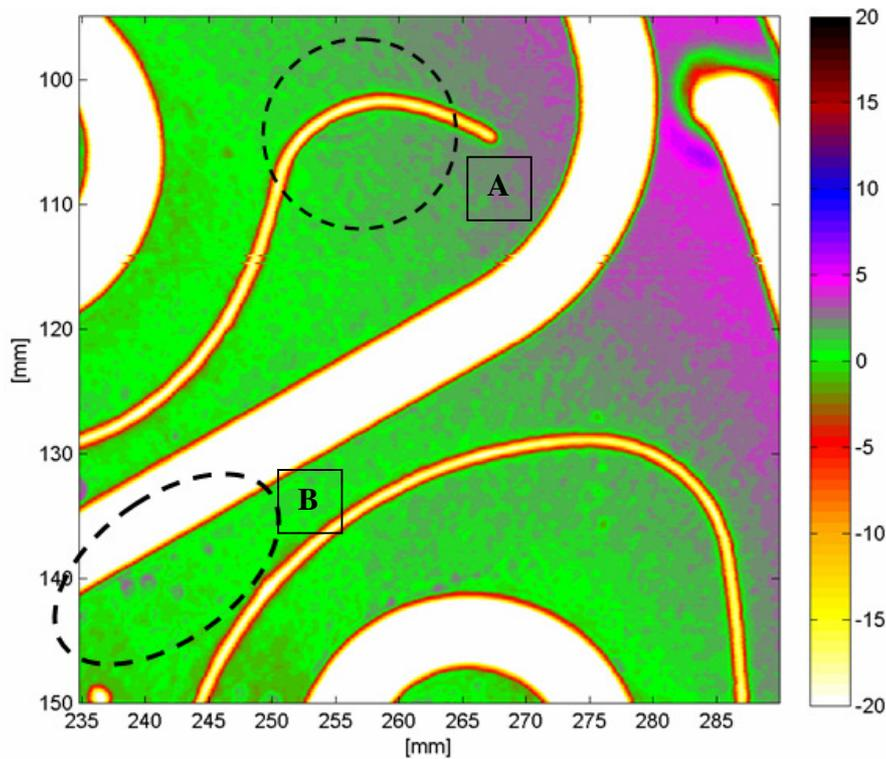
**Figure 6 C-scan using pulse excitation, the scan reveals some defects but they do not show very pronounced.**
