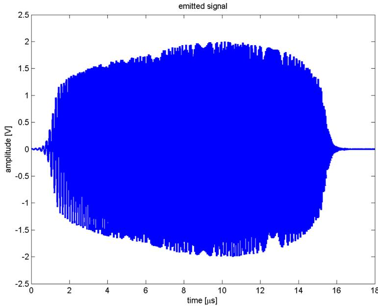
**Figure 3 Optimized sweep signal. The length of the sweep is increased using a quadratic phase shift.**
