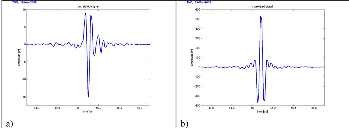
**Figure 4 Transducer response before (a) and after (b) sweep optimization.**
