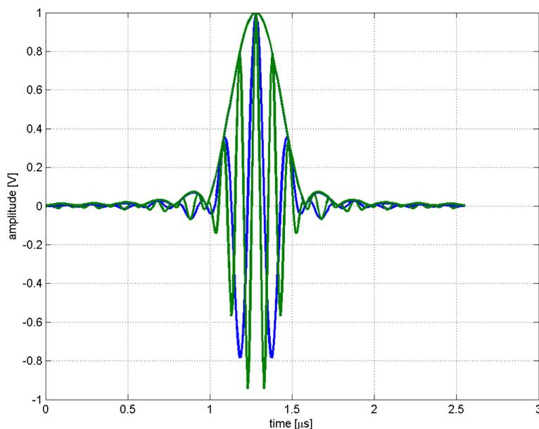
**Figure 1 Comparison of temporal resolution, a 5 MHz signal with 100 % bandwidth yields the same temporal resolution as a 10 MHz signal with only 50 % bandwidth.**
