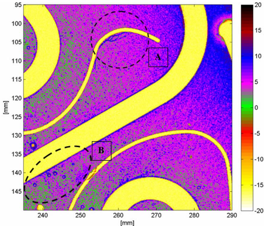
**Figure 7 C-scan using an optimized sweep, the scan reveals much more detail compared to the original C-scan. For example the channel structure (region A) is much better resolved.**
