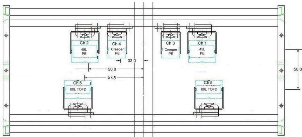
Figure 3 The set-up of scanning frame
