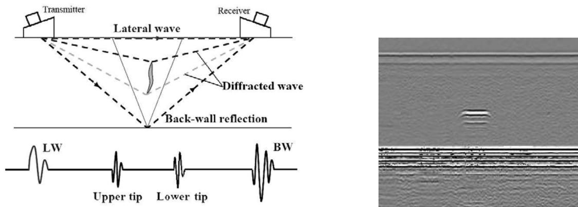
Figure 1 Principle of TOFD technique (left is A-scan; right is TOFD image)
