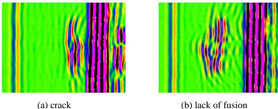
Figure 4 TOFD images of the defects
