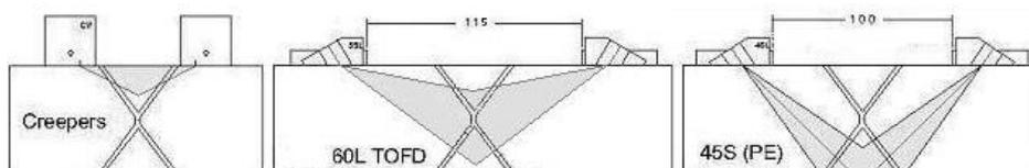
Figure 2 Probes distribution of TOFD scanning
