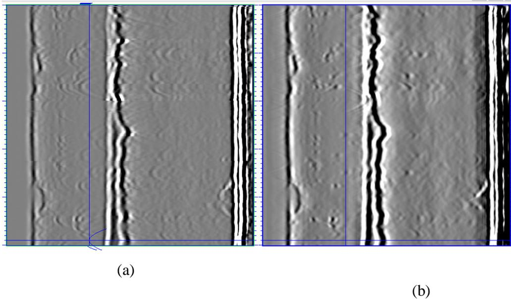
Fig.4 (a)NP-TOFD of block 2#; (b) after SAFT of (a)
