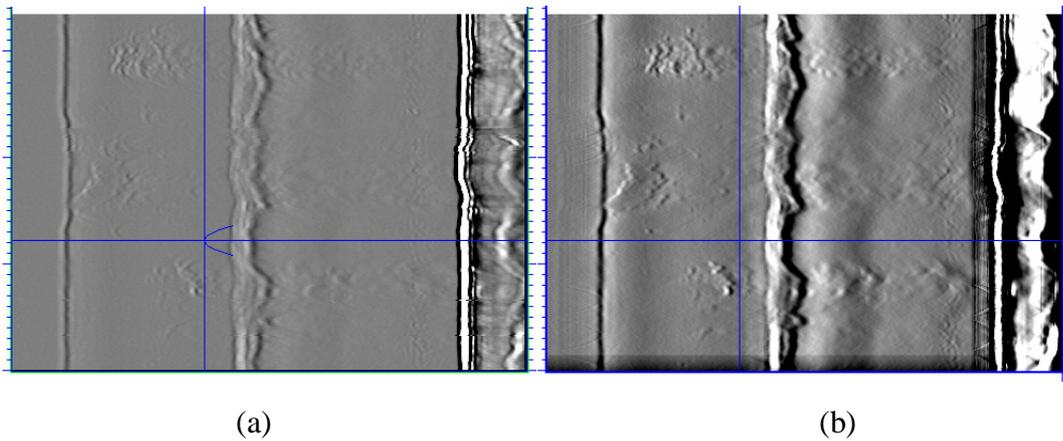
Fig.5 (a)NP-TOFD of block 3#; (b) after SAFT of (a)
