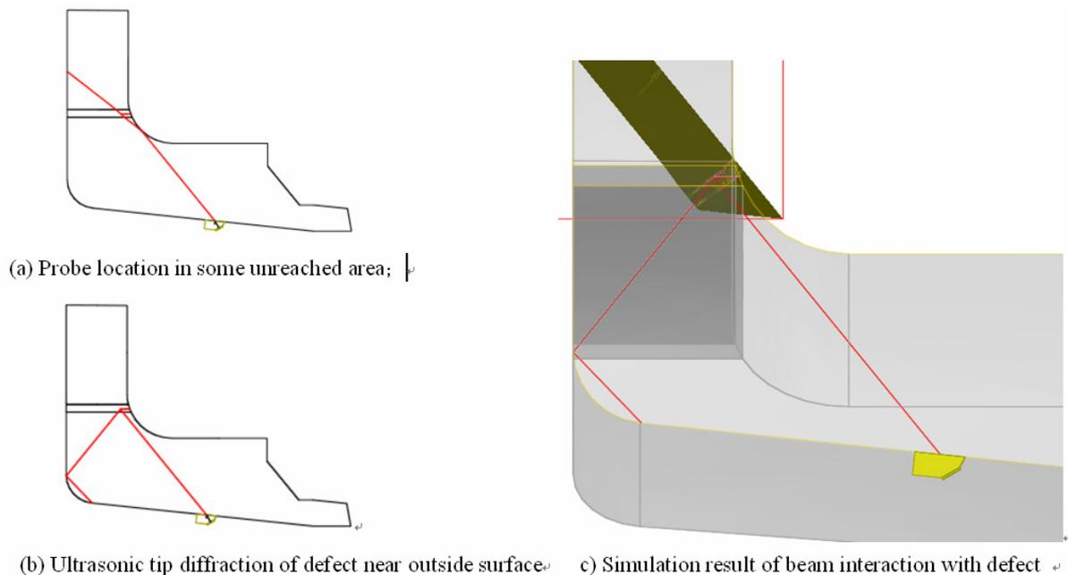
Figure 3 Nozzle to shell weld inspection parameter justification
