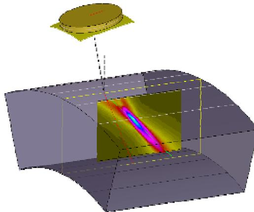
(a) Beam field of an immersion probe in block.
