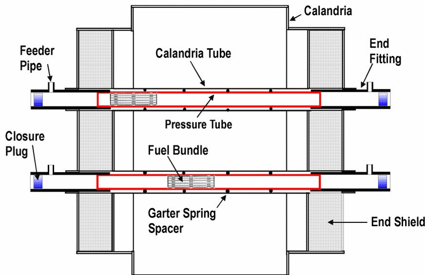
Figure 1 Simplified schematic of CANDU reactor core
