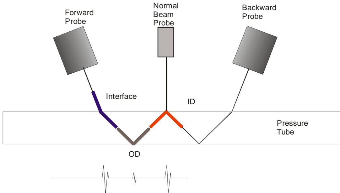
Figure 2 Probe cluster – axial probe pair
