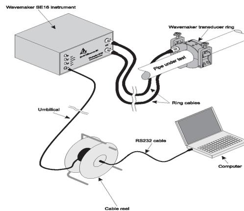
Figure 4. Wavemaker SE16 System Components
