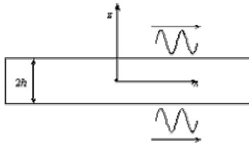
Figure 1. Propagation of a plane harmonic Lamb waves
