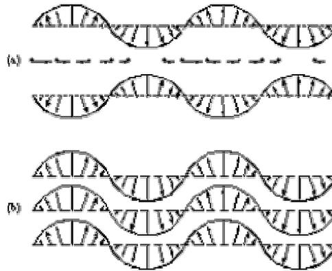
Figure 2. Symmetric (a) and Anti-Symmetric (b) Modes
