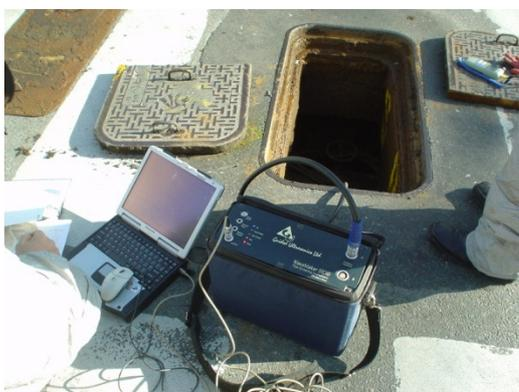
(a) Guided wave sensor for inspection (b) Guided wave inspection
