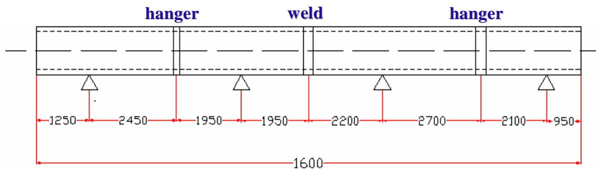
Figure 3. Large Diameter Pipe Specimen Geometrics
