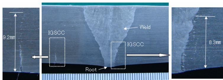
Figure 2. Cross sectional view of the test specimen
