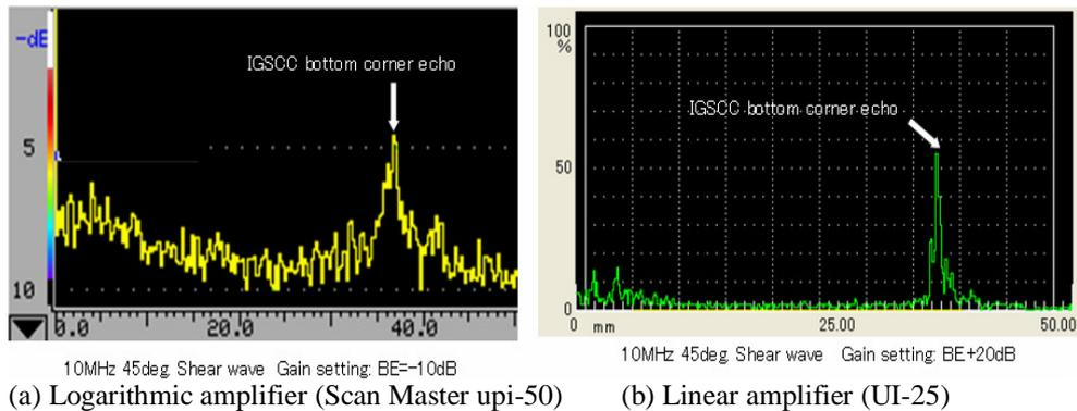
Figure 3. A-scope of IGSCC bottom corner echo
