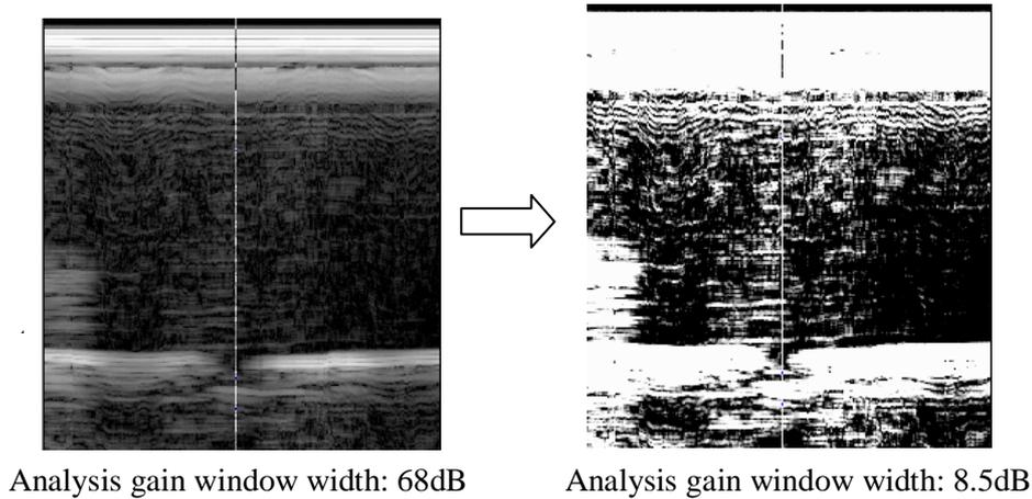
Figure 7. Modification of gain setting to enhance weld geometry
