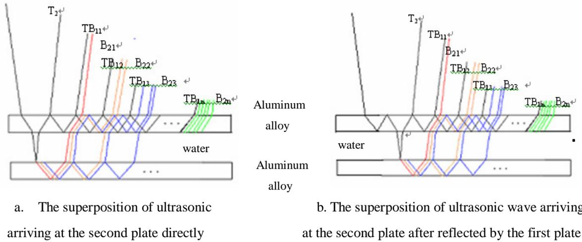
Fig 5 . The routes for ultrasonic superposition
