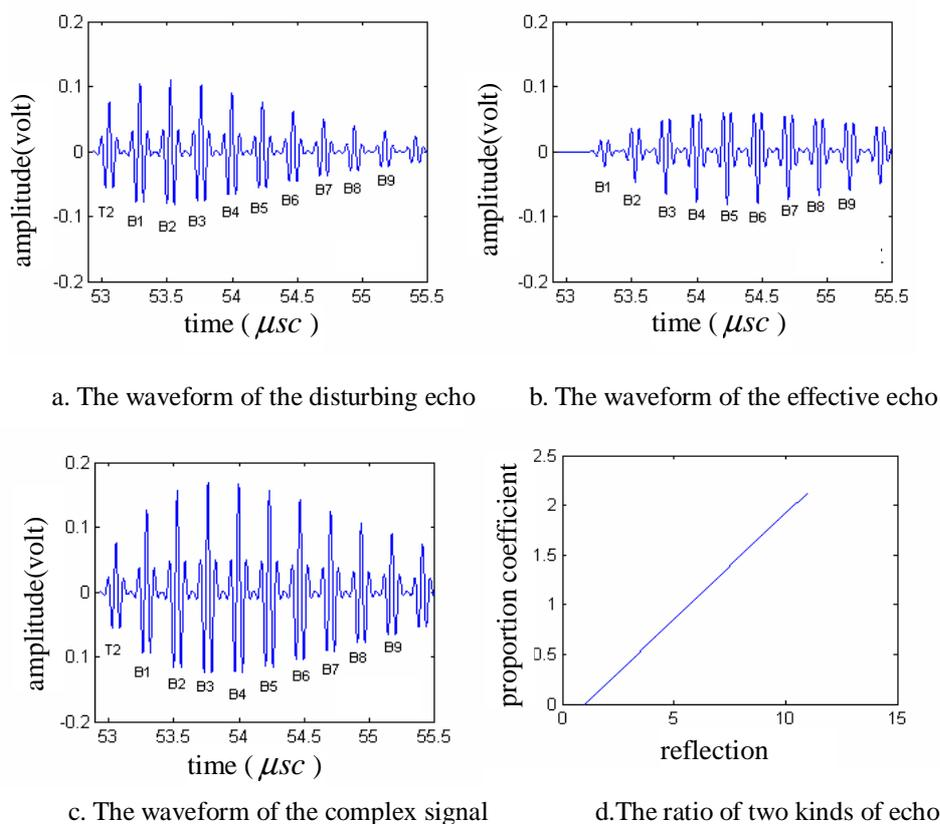
Fig 6 . Simulative waveform of testing the inner weld
