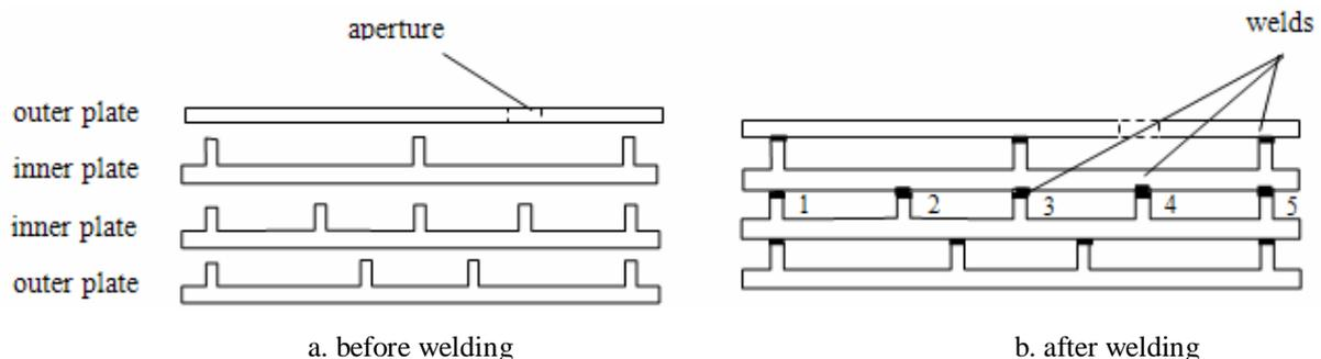
Fig 1. The configuration of multi-layer weld specimen
