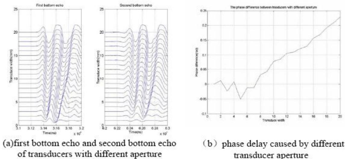
(a) first bottom echo and second bottom echo of transducers with different aperture
