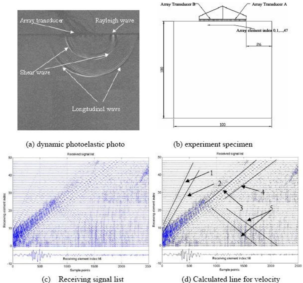
Figure 1. Principle of surface wave velocity measurement and specimen for experiments
