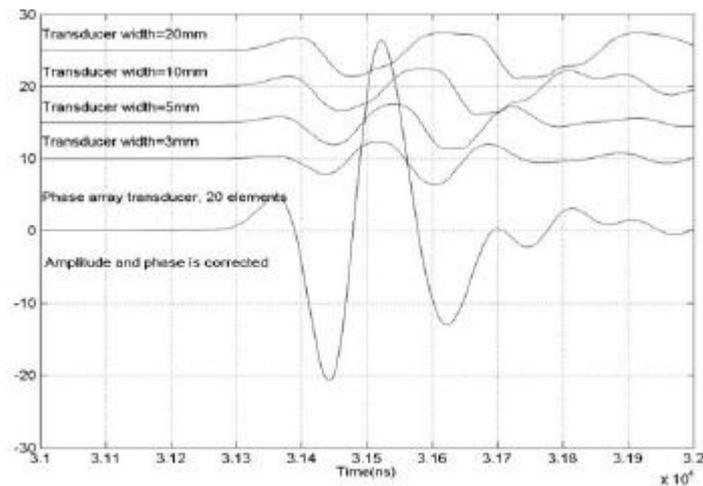
Figure 2. signal from array transducer and from transducers of different width
