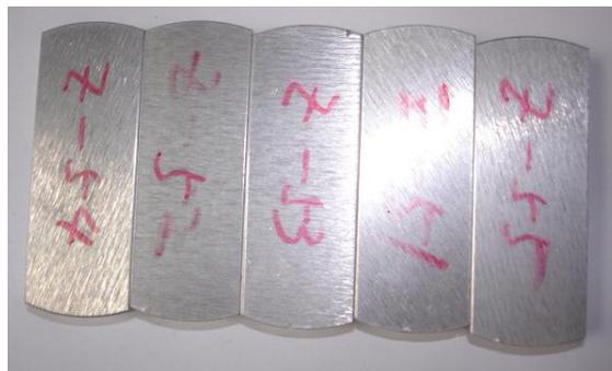
Figure 3 Samples of SiCp/Al with different SiCp content
