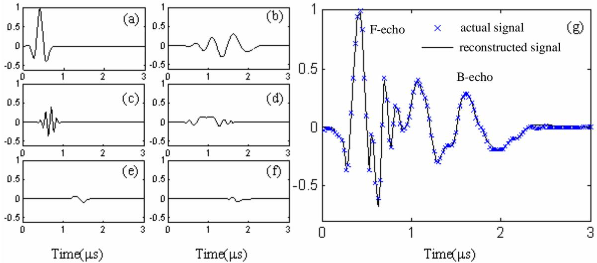
Figure 1. Chirplet decomposition of backscattered signal. (a)- (f) Chirplets decomposed from backscattered signal. (g) Actual (cross) and reconstructed signal (solid line).
