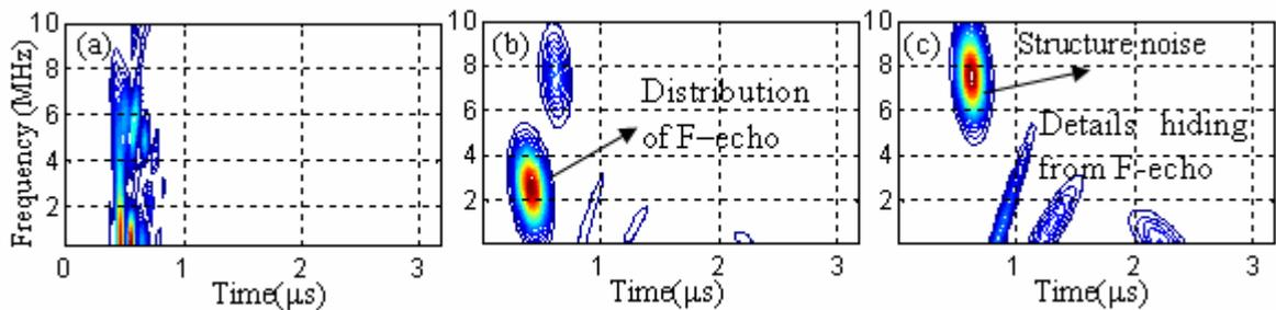
Figure 2. TF representation of ultrasonic signal at position A.
