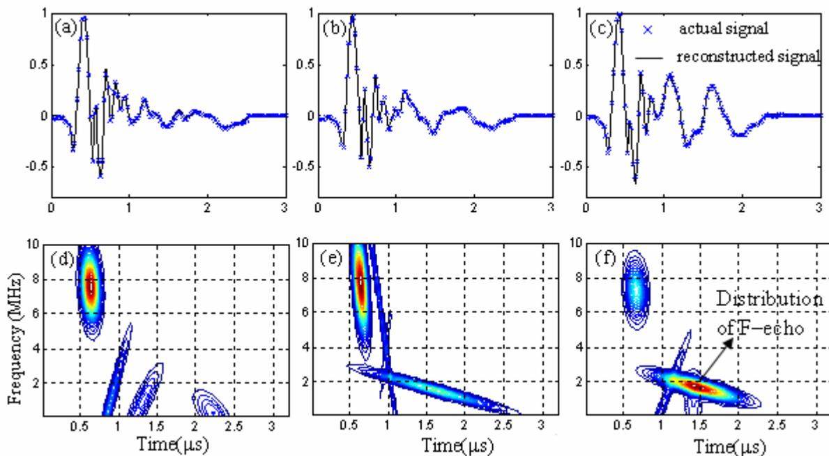
Figure 3. EWVD of signals of severely (A), lightly (B) damaged and undamaged (C) locations. (a), (b), (c) ultrasonic signals of A, B, C. (d), (e), (f) corresponding EWVD.
