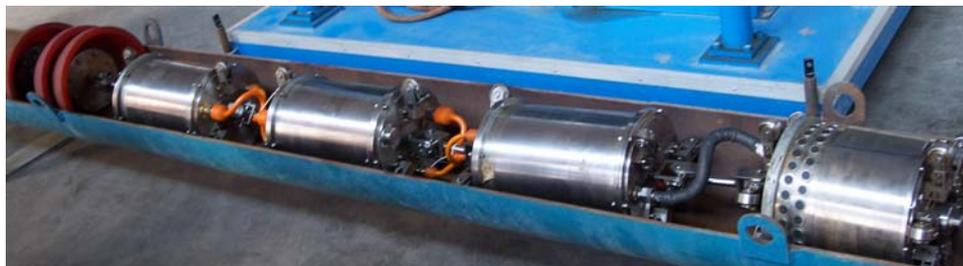
Figure 1 the ultrasonic inspection pig
