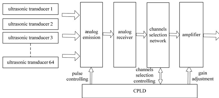
Figure 2 the diagram of ultrasonic analog inspection unit
