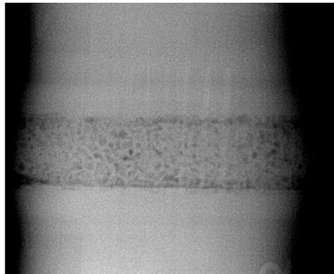
Fig.6. Porosities in 110 mm thick weld (IPS – 4 MeV)
