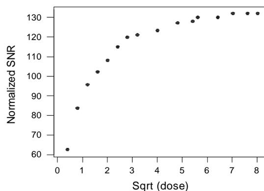
Fig.2. Normalized SNR – IP Type-I – IPS with Ir-192.
