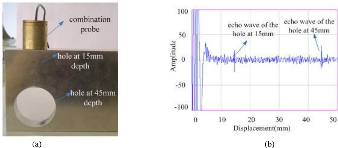
Fig.6 Result of testing the hole defection inside of the steel. (a) Sample with hole defection testing with combination probe. (b) Result of the measurement with combination probe in EMAT channel
