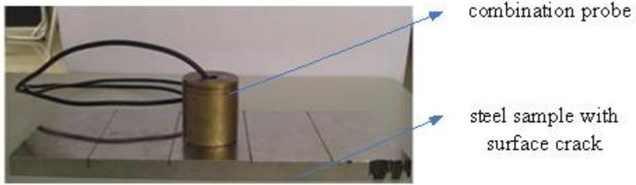
Fig.3. Steel sample with different depth surface crack testing with combination probe
