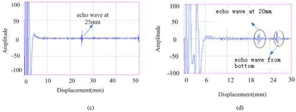
Fig.5. Result of testing the steel plate simulation of the thickness reduction in EMAT channel with combination probe. (a). Testing the steel sample simulation thickness reduction with combination probe. (b). Testing result from 20mm location in EMAT channel. (c). Testing result from 25mm location in EMAT channel. (d). Testing result from location of thickness reduction in EMAT channel.
