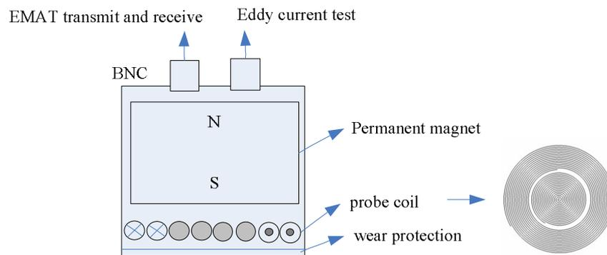
Fig. 1. Structure of the combination probe
