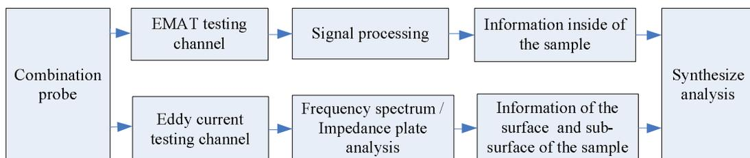
Fig.2. System framework of the combination testing method
