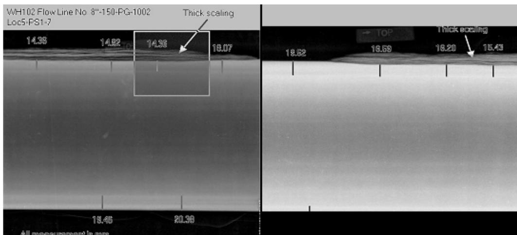
Figure 4. Corresponding digital images show the scaling and remaining wall thickness
