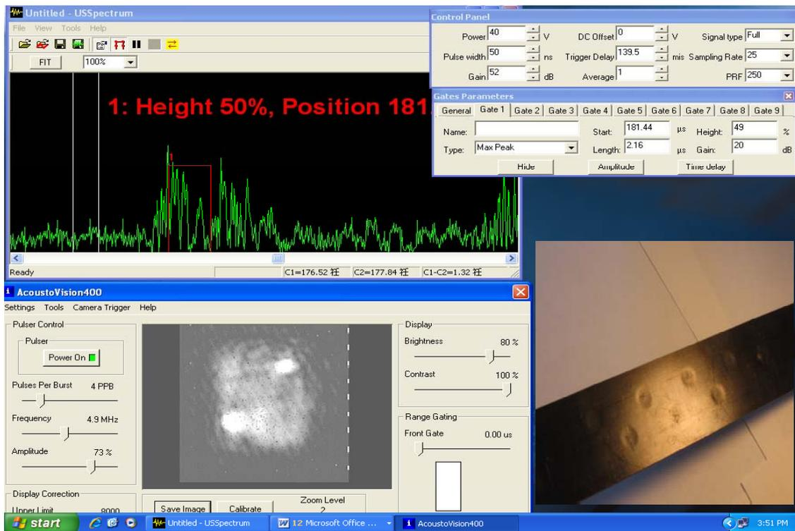
FIGURE 7. Real-time ultrasonic A-scan and image of the damaged area from low-velocity impact of energy 28J.
