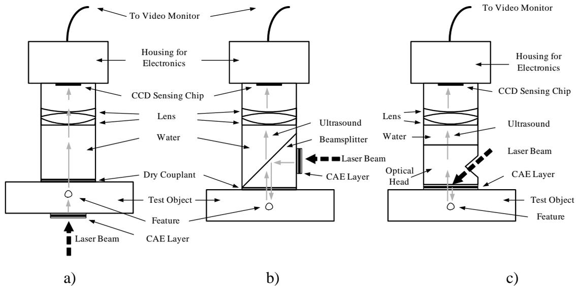
**Figure 8:** Ultrasonic imaging system diagram using laser-based ultrasound generation: a) pulse-echo mode with beamsplitter, b) through-transmission mode with beamsplitter, and c) pulse-echo mode using an optical head.
