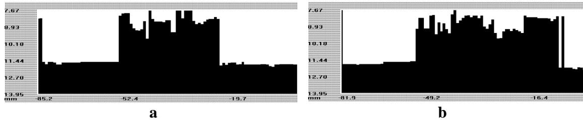
FIGURE 6. B-scan images of the damaged areas from low-velocity impacts of energy 22J (a) and 28J (b).
