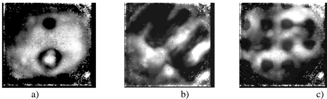
Figure 9: Images of subsurface defects in pulse-echo mode with a laser-based ultrasonic source.
