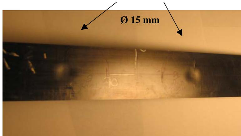
**FIGURE 4** Composite coupon with two damaged areas from the low-velocity impacts.
