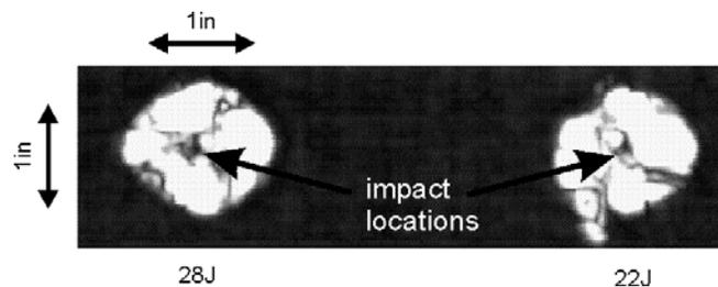
**FIGURE 5.** C-scan of the impacted cross-ply coupon in the damaged area (two hit-points with the energy of 28 J and 22J).
