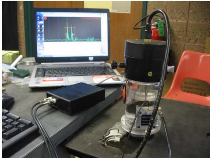
**FIGURE 2.** Integrated dual-channel inspection system.
