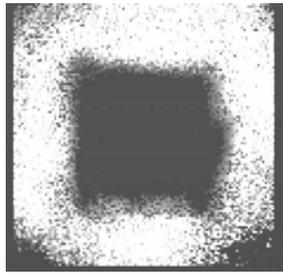
Figure 10: Image of a square-pillow defect in a unidirectional composite panel, using a laser-based ultrasonic source and in through-transmission.
