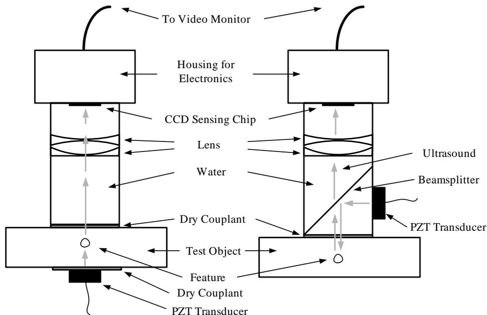
**FIGURE 1.** System diagram of the real-time, dry-coupled, high-resolution ultrasound imaging system using PZT generation: (a) through-transmission mode; (b) pulse-echo mode.
