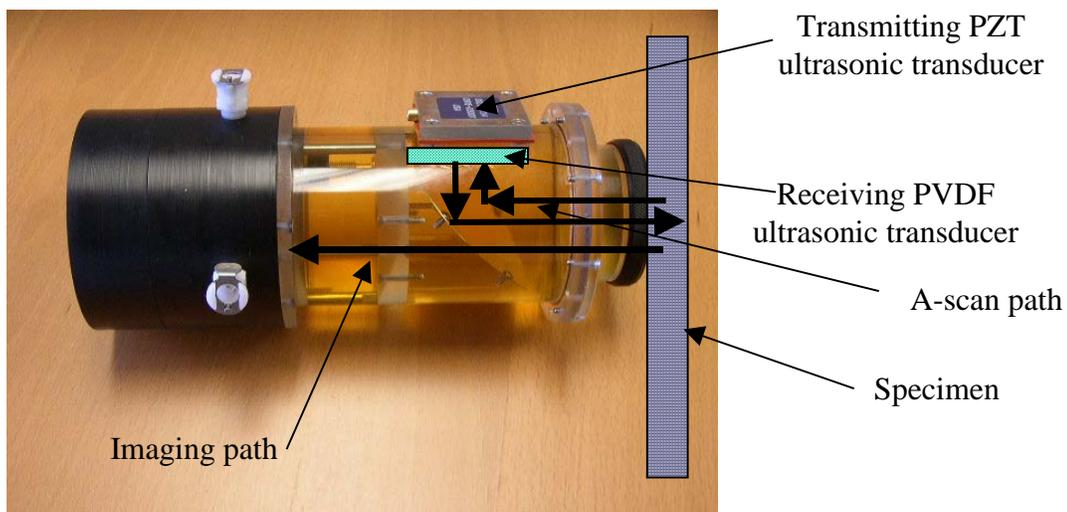
**FIGURE 3.** Transmitting/receiving configuration of the A-scan and imaging channels.
