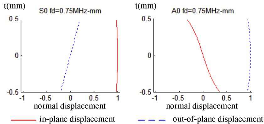
Figure 5 wave structure for various points on the S0 mode and A0 mode of guide waves in aluminum plate
