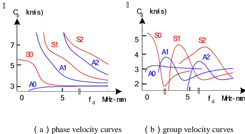
Figure 1 the dispersion curves of guided waves in the aluminum ,  $C_L=6.37\text{km/s}$  ,  $C_T=3.16\text{km/s}$
