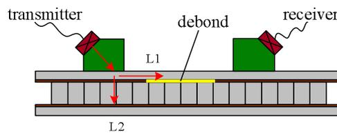
Figure 2 the sketch of guided waves in skin-honeycomb core sandwich plate
