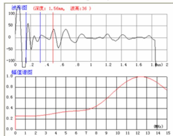
Fig 2 waveform and spectrum produced by the apodization probes
