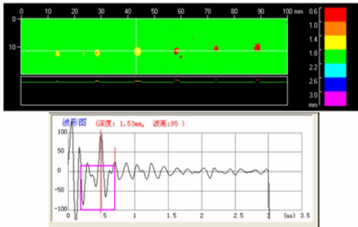
Fig3 depth image (the upper) and a time-domain waveform of the image (the below)
