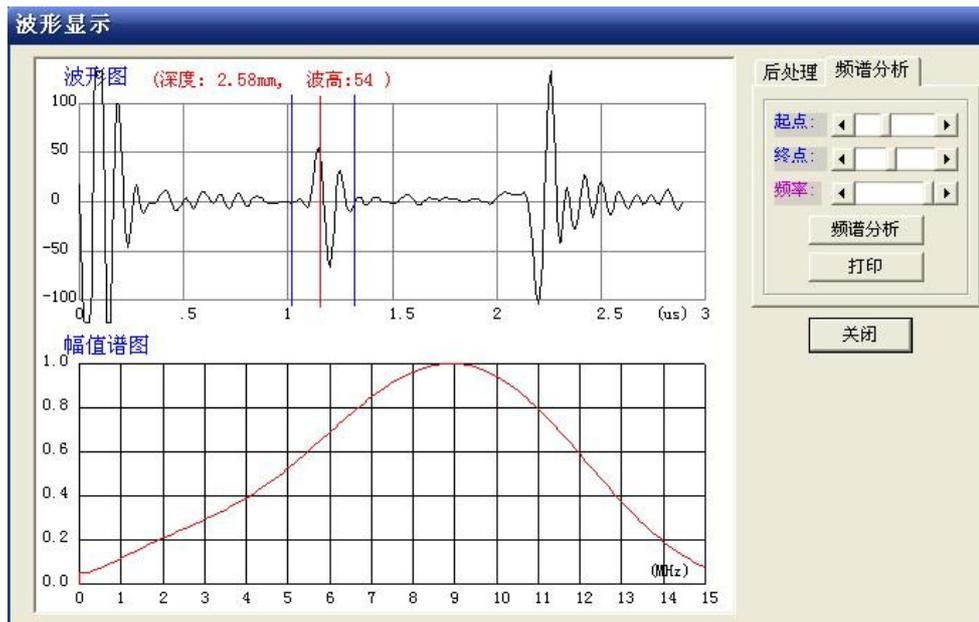
Figure 4. Transducer's wave and frequency
