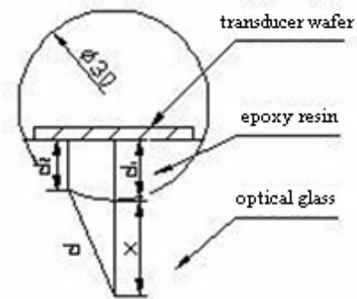
Fig 3 sketch map of the simulated experiment sample
