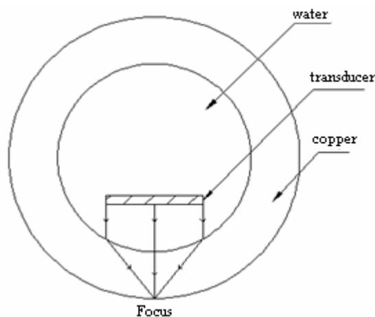
Fig 2 sketch of principle of focus
