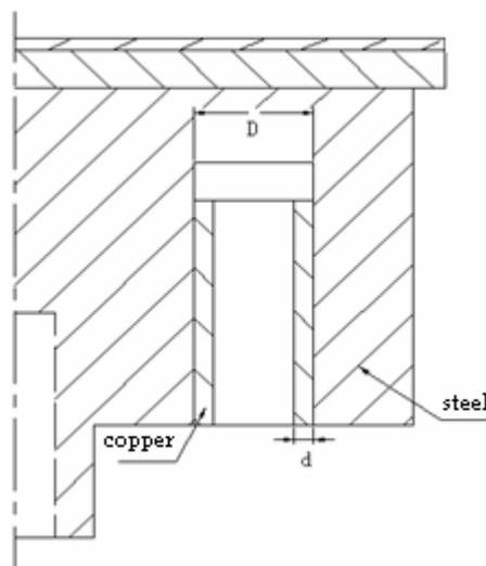
Fig 1 sketch map of bimetal rotor
