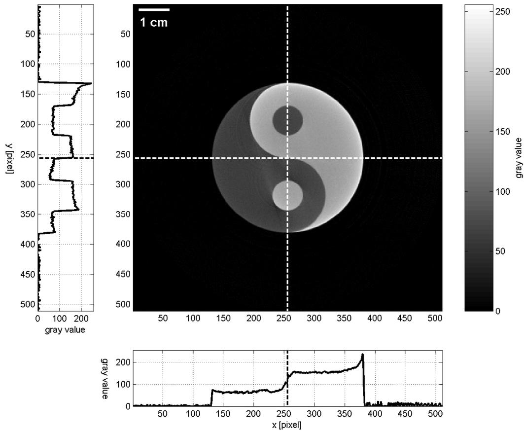
Figure 2: Central slice of simulated object Yin and Yang and corresponding line profiles.
