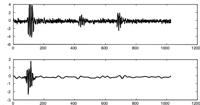
Figure 1 - *Debauchee 8 DWT filtering of a 5mm circle signal*
