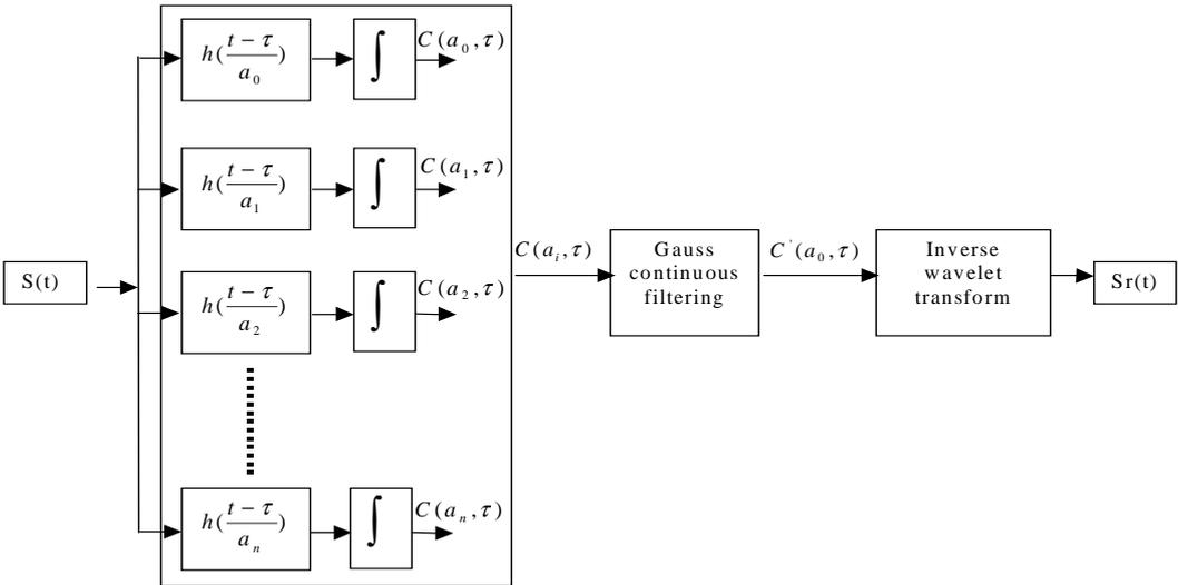
Figure 2 - Continuous filter bank of S(t)
