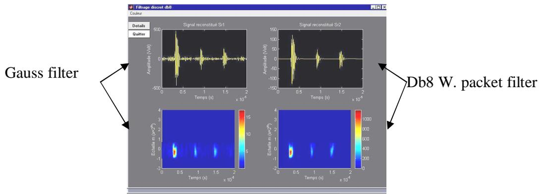
Figure 4 - Wavelet packet filter
