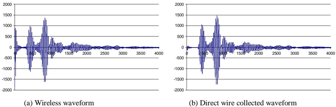
**Figure 6.** Comparison of ultrasonic guided wave data collected by (a) the wireless SHM device, and (b) the direct wire connected instrument.
