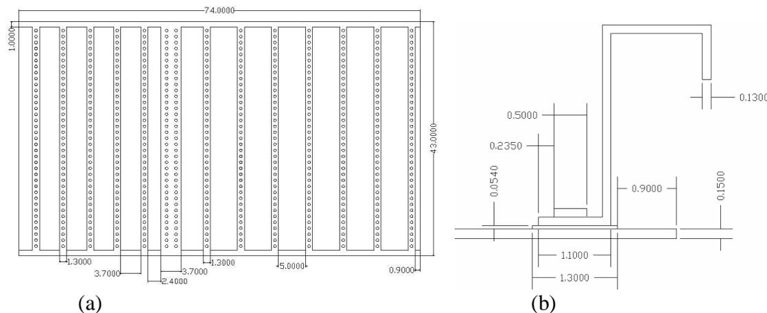
**Figure 1.** Wing skin structure (a) overview of the rivet row sketch (b) typical geometry of a stiffener riveted to the skin (all the scales are in cm)
