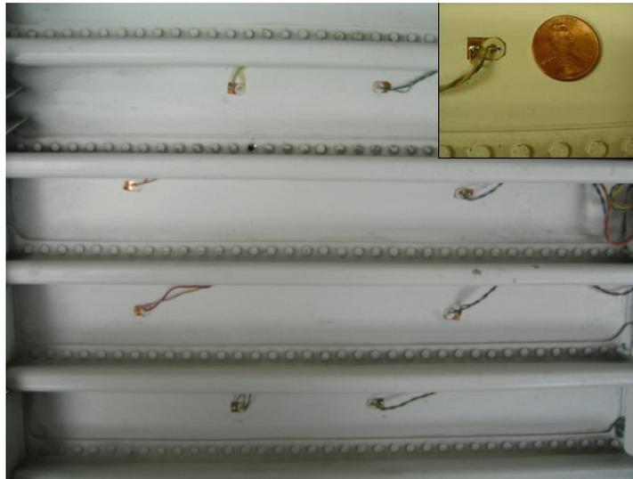
**Figure 2.** Eight element PZT array mounted on the wing panel. The image on the top right corner shows the transducer size compared with a coin.
