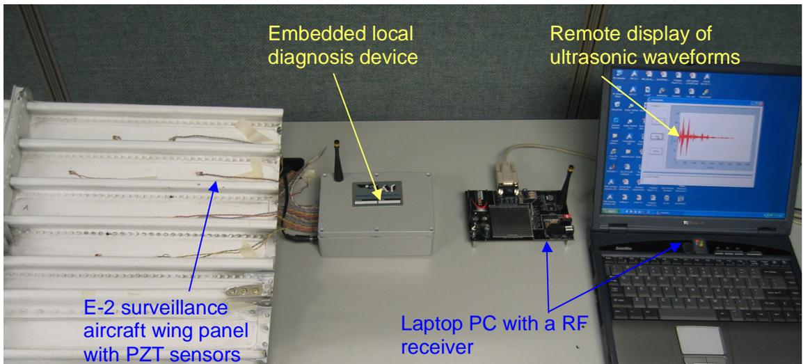
**Figure 5.** Embedded ultrasonic data acquisition and wireless transfer system for an E-2 wing panel inspection.
