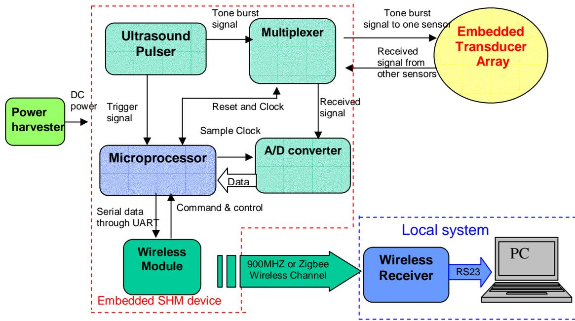
**Figure 3.** Diagram of the embedded ultrasonic structural health monitoring system
