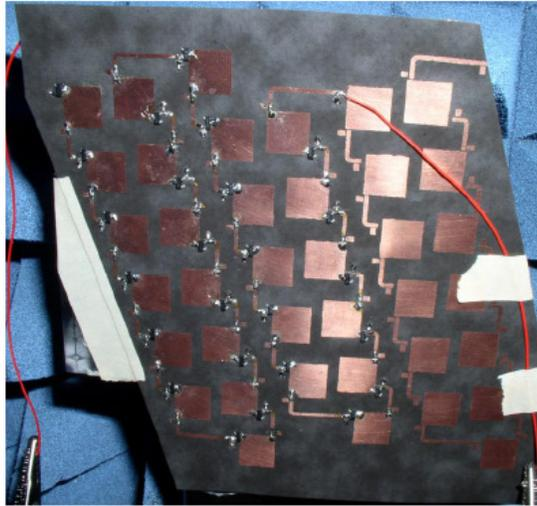
**Figure 4.** X-band microwave rectenna for wireless powering the on-board electronics
