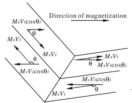
Fig.4 Value on a direction of magnetic moment of magnetic domain
