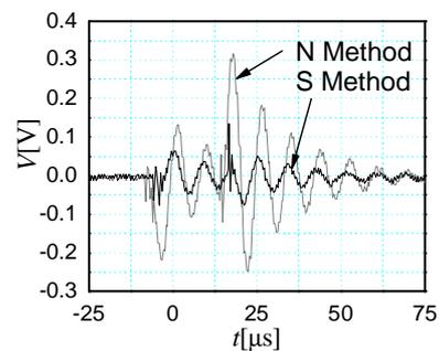
Fig.3 Induced waveform without amplifier
