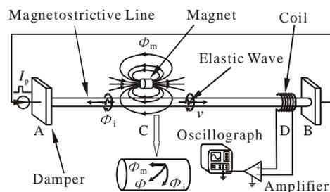
Fig.1 The principle of magnetostrictive line sensor
