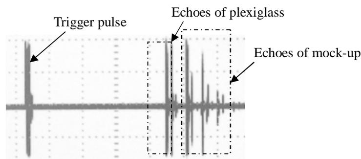
Figure 11 waveforms gained using the rotated acoustic mirror
