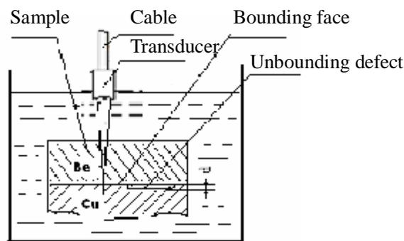
Figure 2 diagrammatic sketch of water immersion ultrasonic test
