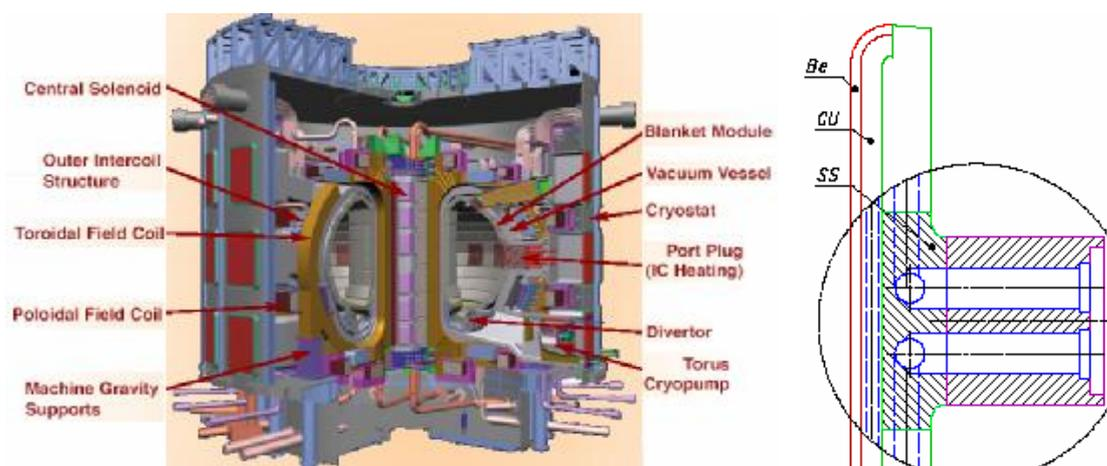
Figure 1. Structure of ITER and the First Wall
