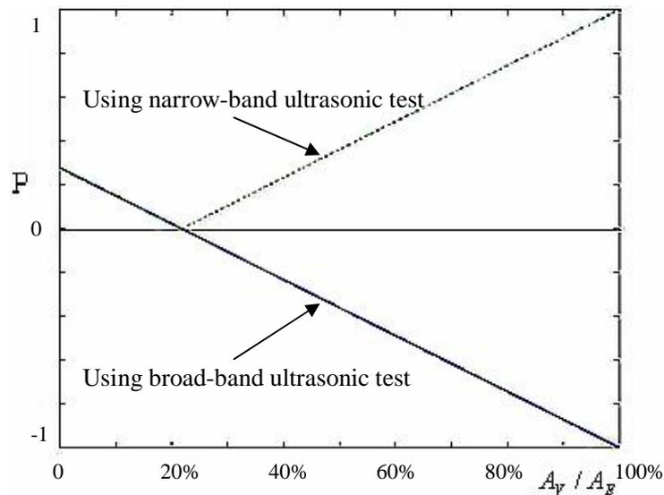
Figure 6 relations of echo amplitude and unbounding ratio
